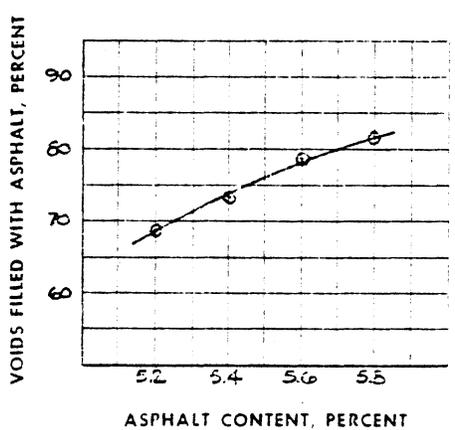
Figure B-4. Results of Marshall tests on Lone Star B mix.
