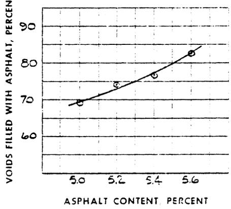
Figure B-2. Results of Marshall tests on Shadwell mix.
