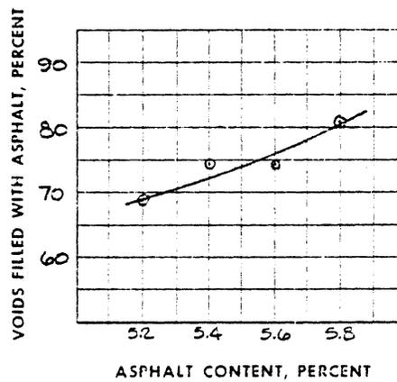
Figure B-3. Results of Marshall tests on Lone Star A mix.
