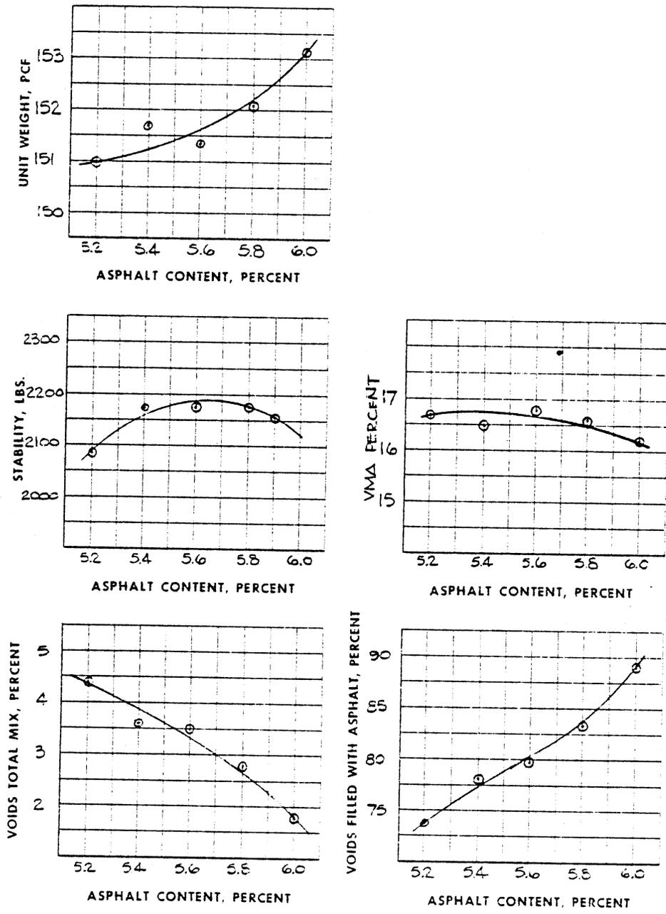
Figure B-1. Results of Marshall tests on Red Hill mix.
