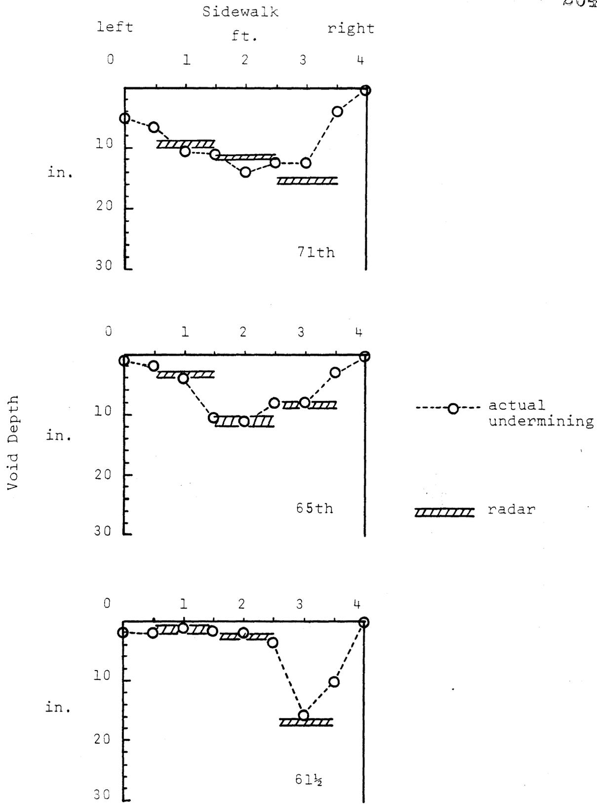
Figure 9. Comparison of some radar results with actual undermining profile. Metric conversion: 1 inch = 25.4 mm.
