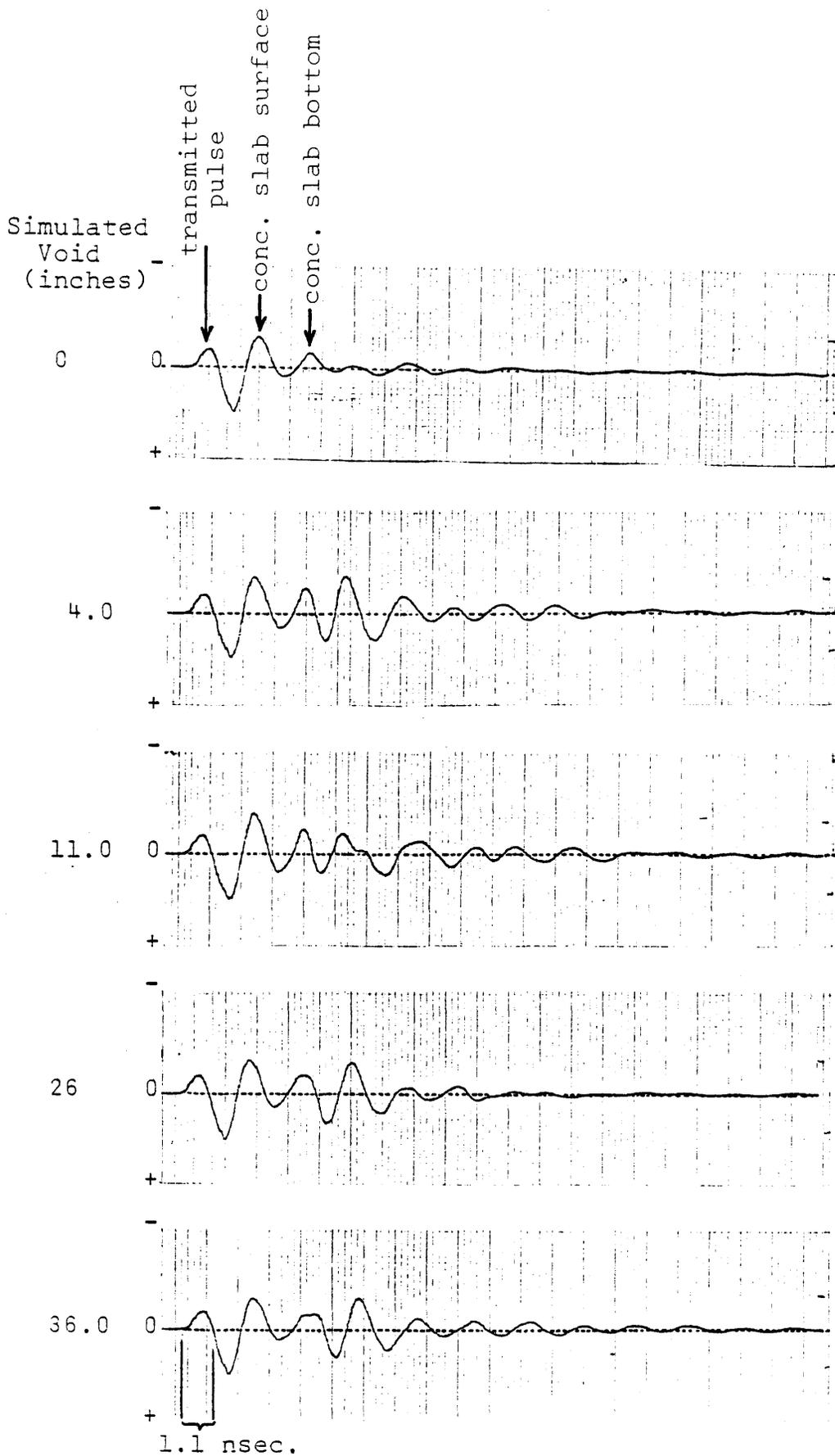
Figure 5. Radar echo waveforms observed for the simulated sidewalks of different void sizes underneath the concrete slab. Metric conversion: 1 inch = 25.4 mm.
