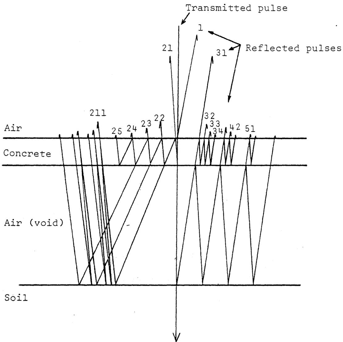
Figure 8. Propagation of radar pulses in an air/concrete/air/soil system.
