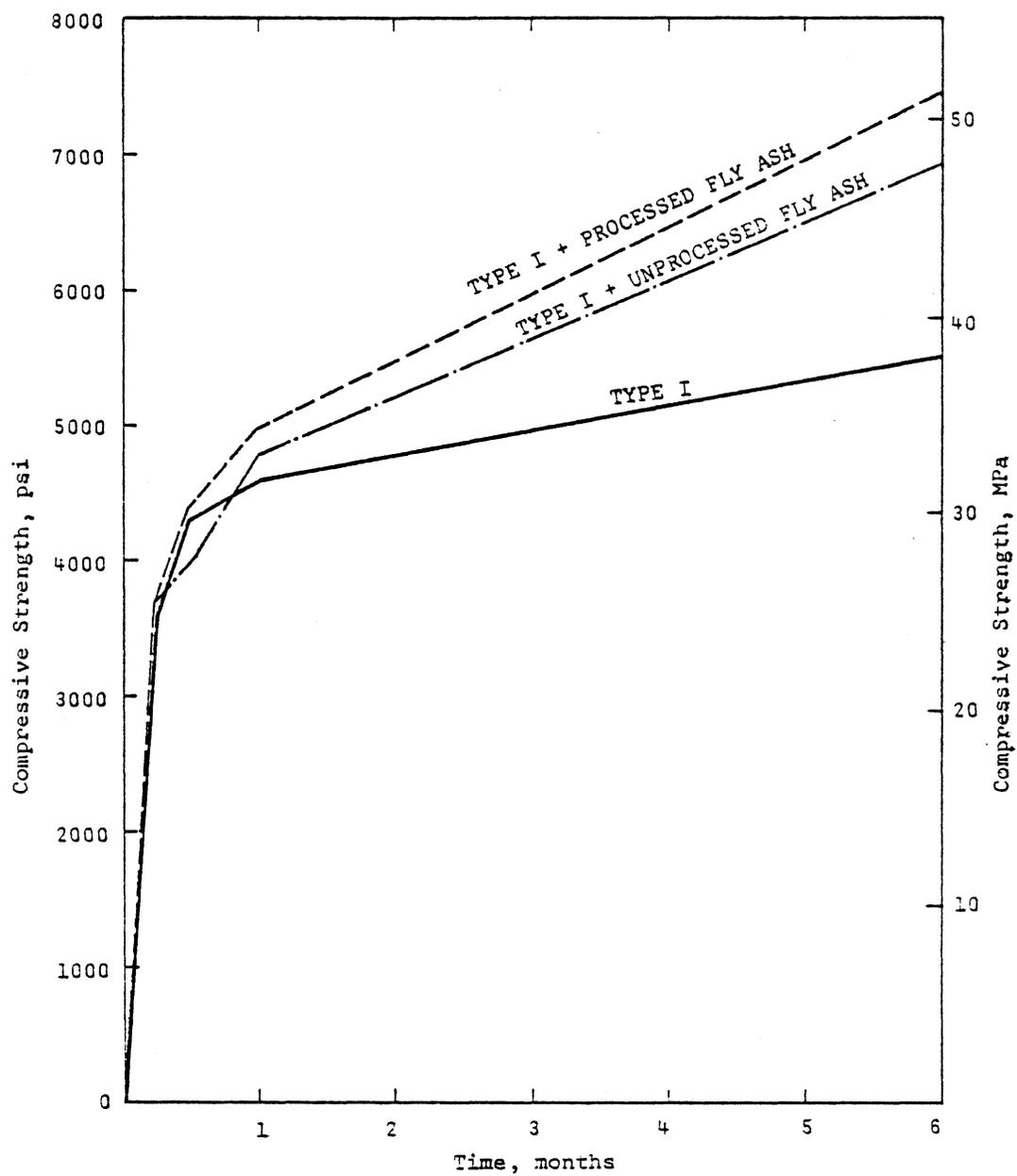
Figure A-1. Strength-age relationship of A3 concrete mixtures.
