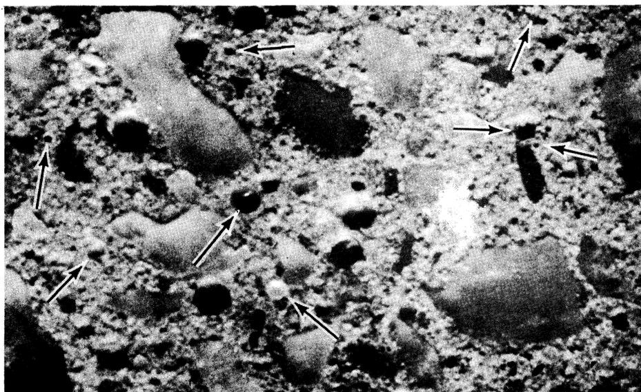
Figure 5. At top, polished surface (24x); bottom, etched surface (45x). Fly ash particles are indicated by arrows; remaining voids are assumed to be air bubbles.
