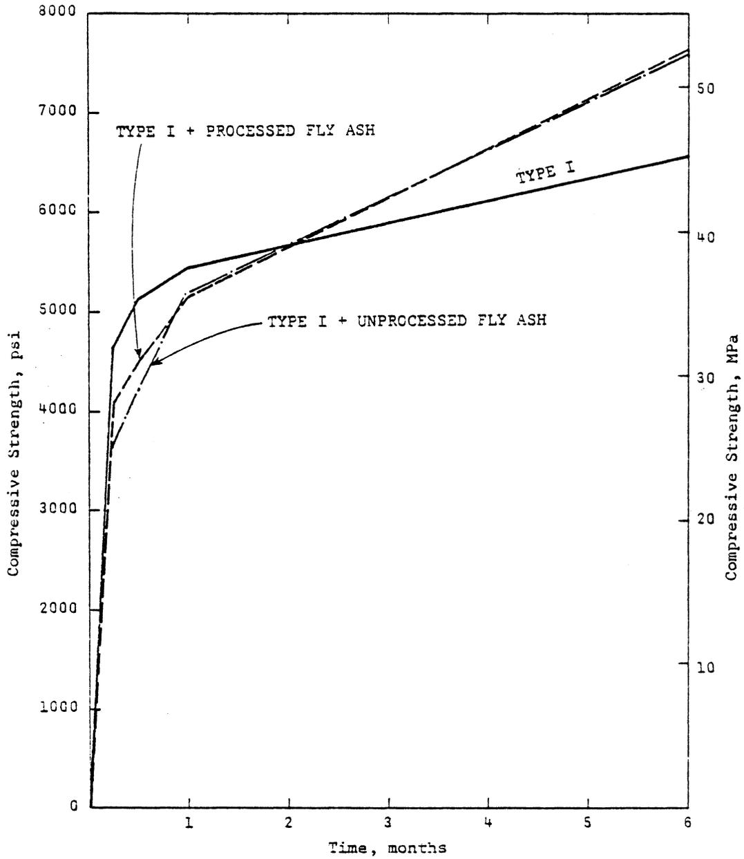
Figure A-2. Strength-age relationships of A4 concretes.
