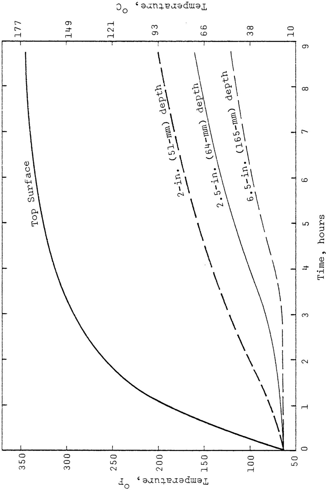
Figure 21. Temperature changes in bridge deck slab.
