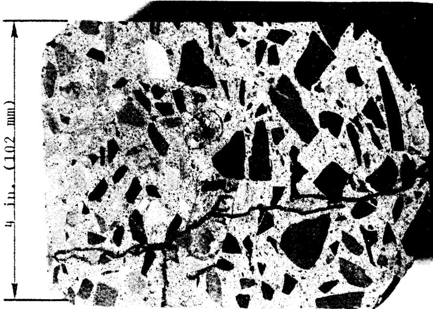
Figure 16. Core through overlay and raked base layer.
