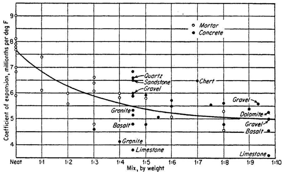
Figure 11. Thermal coefficients of expansion of neat cements, mortars, and concretes.<sup>(2)</sup>
