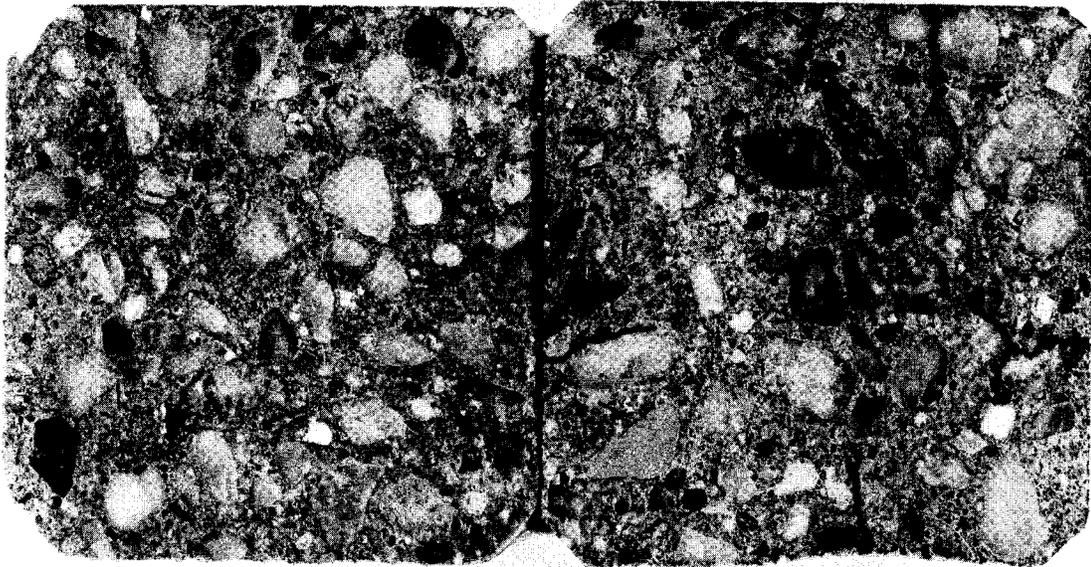
Figure 12. Polished sections from unheated (left) and heated (right) 3 x 3 x 11 in. (76 x 76 x 279 mm) prisms.
