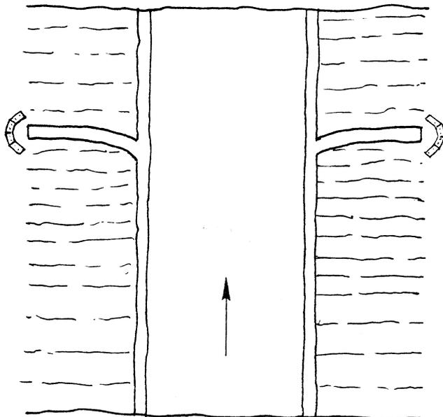
Figure 9. Plan view of fill being constructed. Note the berms at edge of fill and the temporary downdrains.
