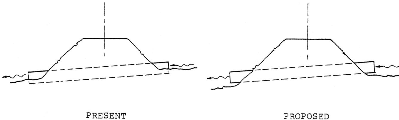
Figure 8. Present and proposed placement of drain pipe under fills.
