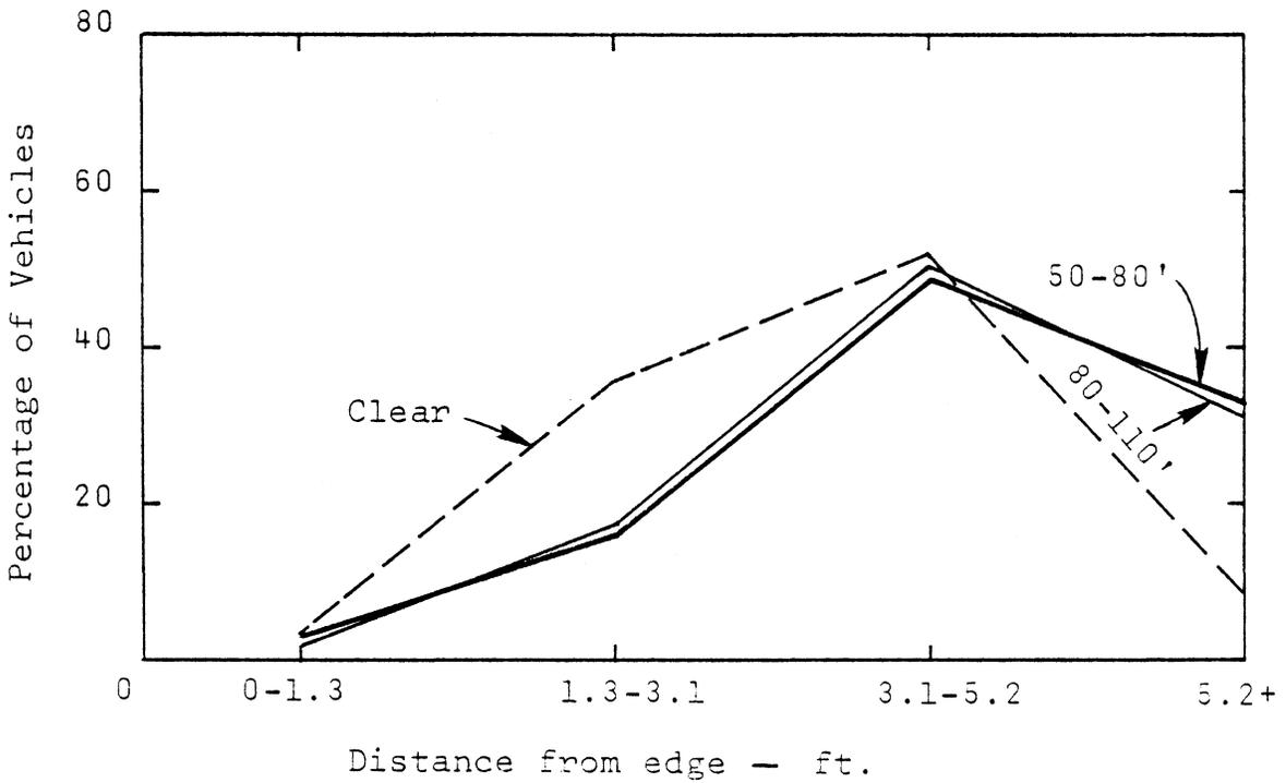
Figure 13. Placement interval from pavement edge for cars at night - after period. (1 ft. = 0.30 m)
