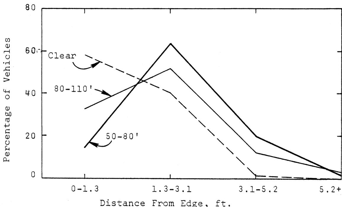
Figure 14. Placement interval from pavement edge for tractor-trailers at night - after condition. (1 ft. = 0.30 m)
