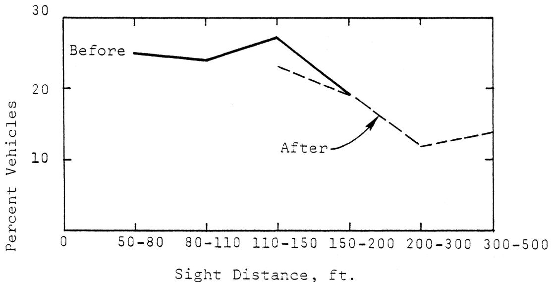
Figure 7. Percentage of vehicles in lane 1 below 3 seconds, daylight. (1 ft. = 0.30 m)
