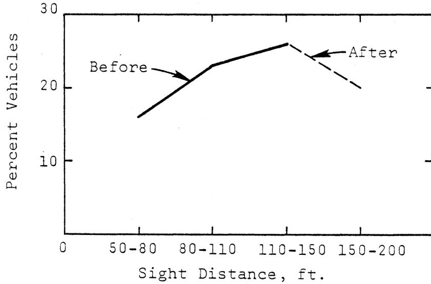
Figure 8. Percentage of vehicles in lane 2 below 3 seconds, daylight. (1 ft. = 0.30 m)
