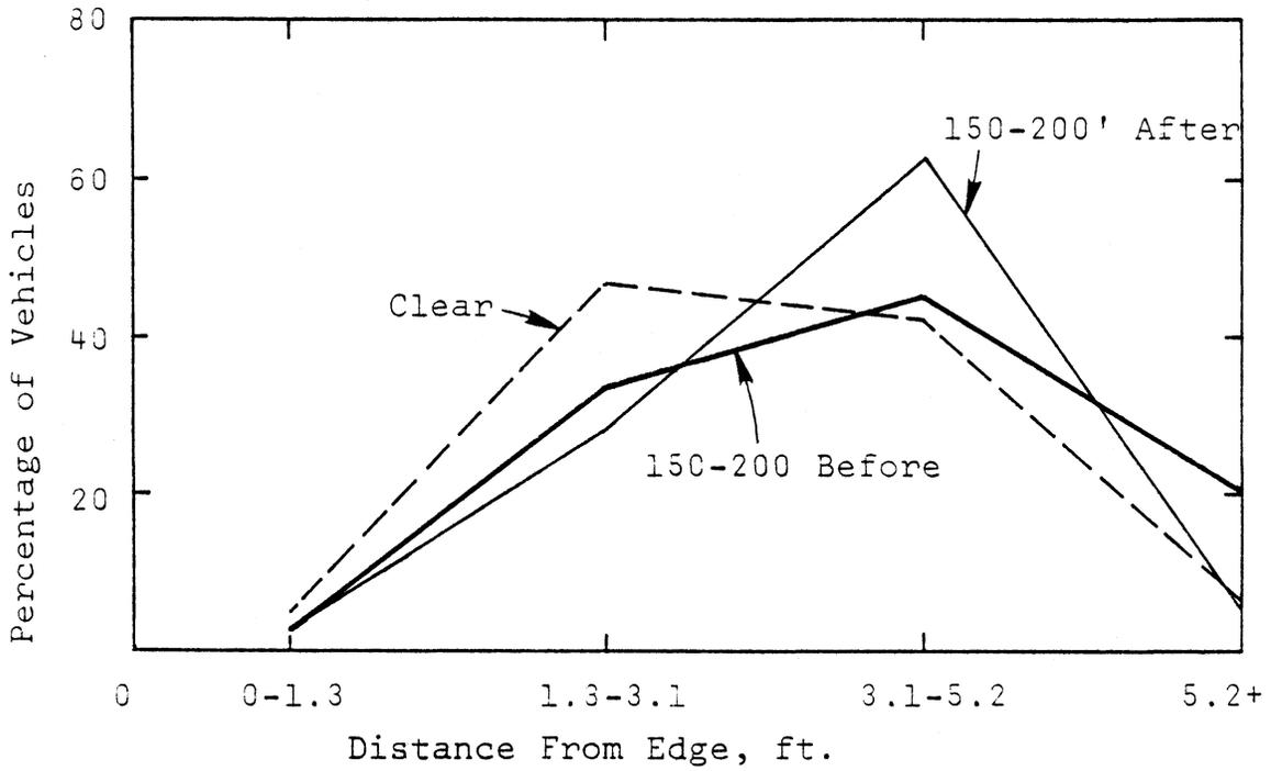
Figure 12. Placement interval from pavement edge for cars during daylight. (1 ft. = 0.30 m)
