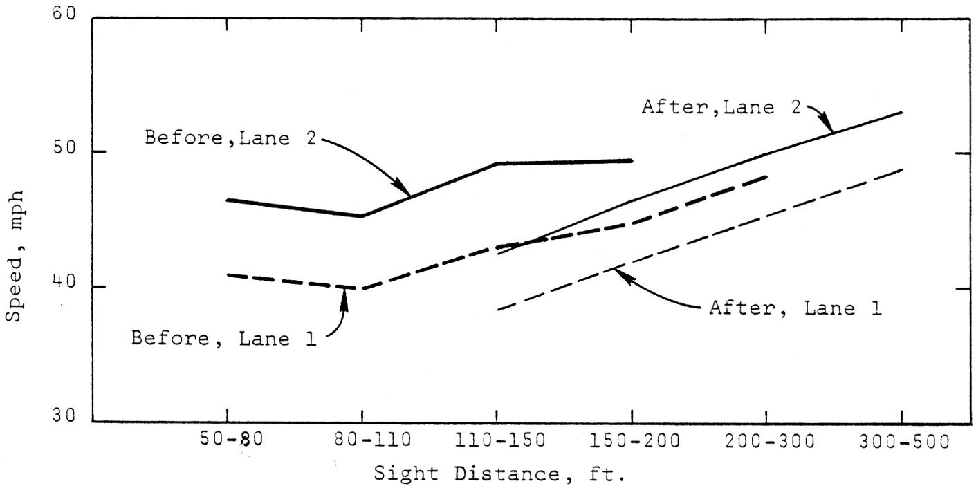
Figure 4. Mean car speed versus sight distance for daylight fog conditions. (Note: 1 mph = 1.6 kmh; 1 ft. = 0.30 m)
