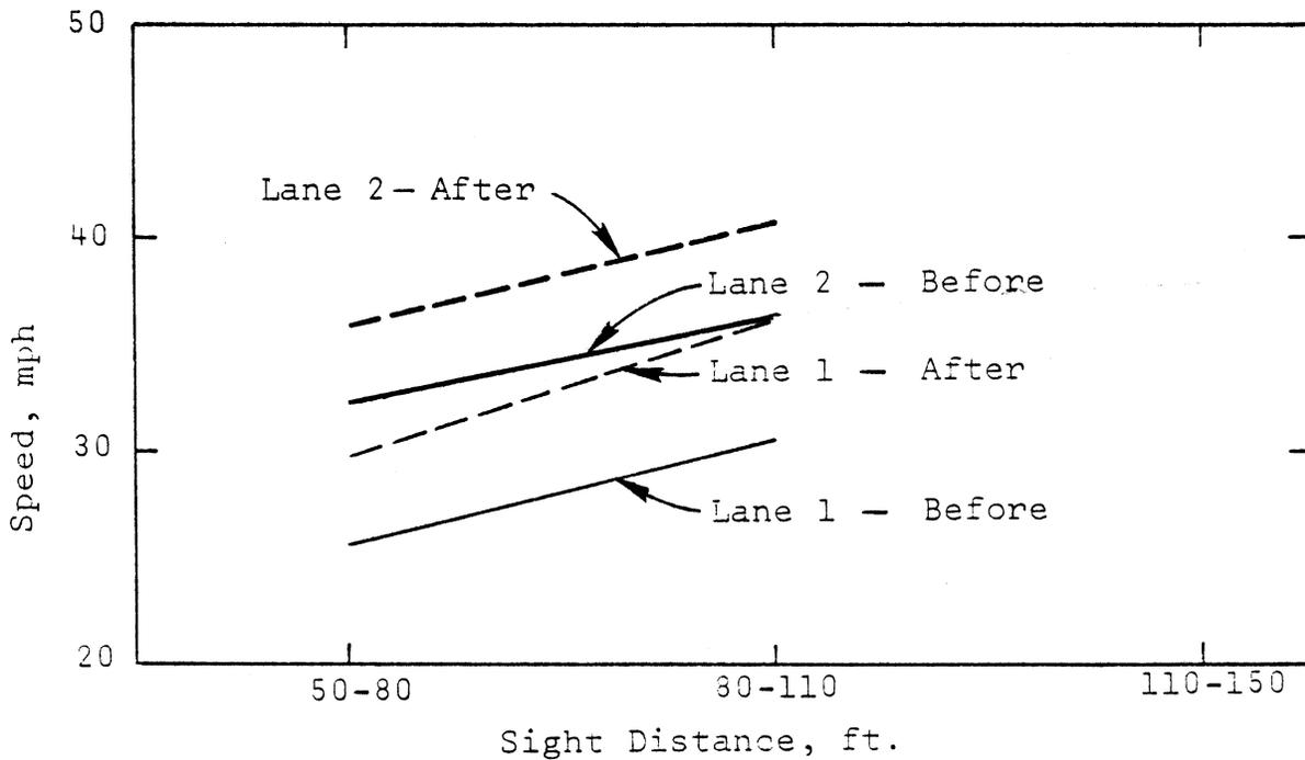
Figure 5. Mean car speed versus sight distance for nighttime fog conditions. (Note: 1 mph = 1.6 kmh; 1 ft. = 0.30 m)
