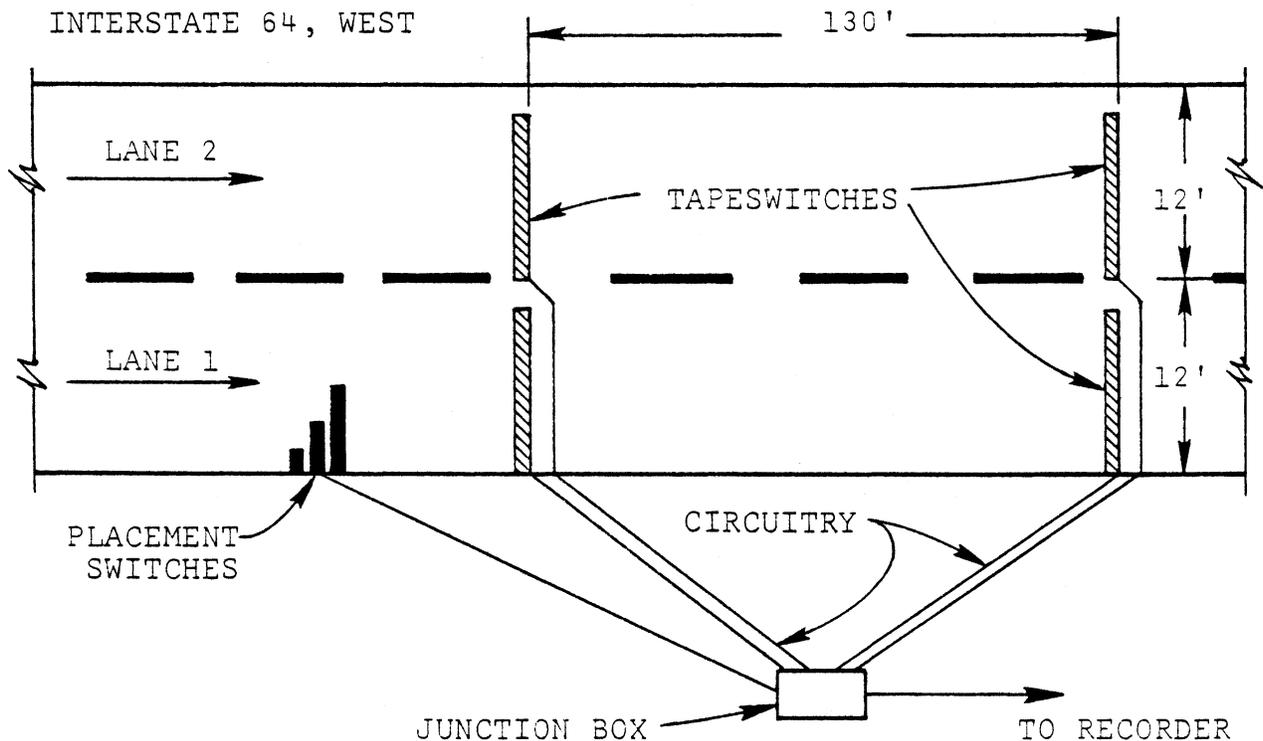
Figure 3. System of tapeswitches used for data collection.
