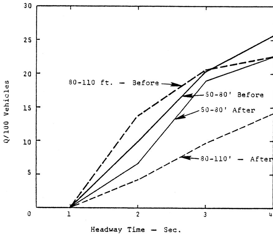
Figure 11. Vehicle queuing for headway cutoff time shown - nighttime (1 ft. = 0.30 m).
