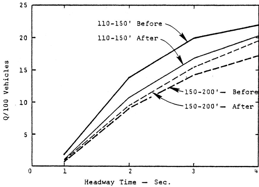
Figure 10. Vehicle queuing for headway cutoff time shown - daytime. ( 1 ft. = 0.30 m).
