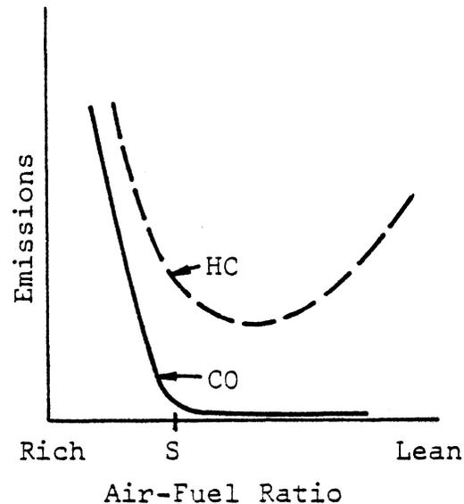
Figure 3. Well-established relationship between exhaust emissions and air-fuel ratio. (After Brinkman. (8))
