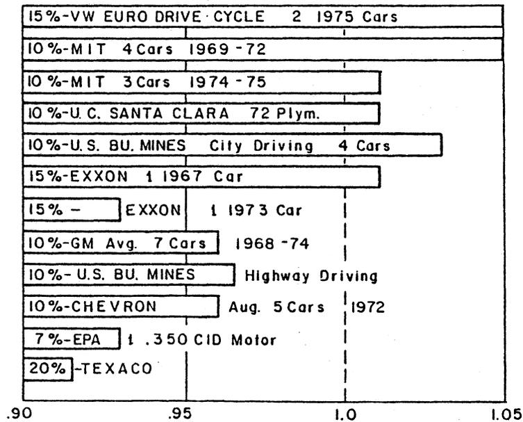
Figure 2. Fuel economy for vehicles and engines operated on various percentages of methanol as compared to gasoline and reported by various laboratories. (After Reed (7).)
