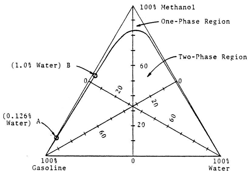
Figure 6. Equilibrium phase diagram for system: Methanol, water, and gasoline at 76°F. [After API.(10)]
