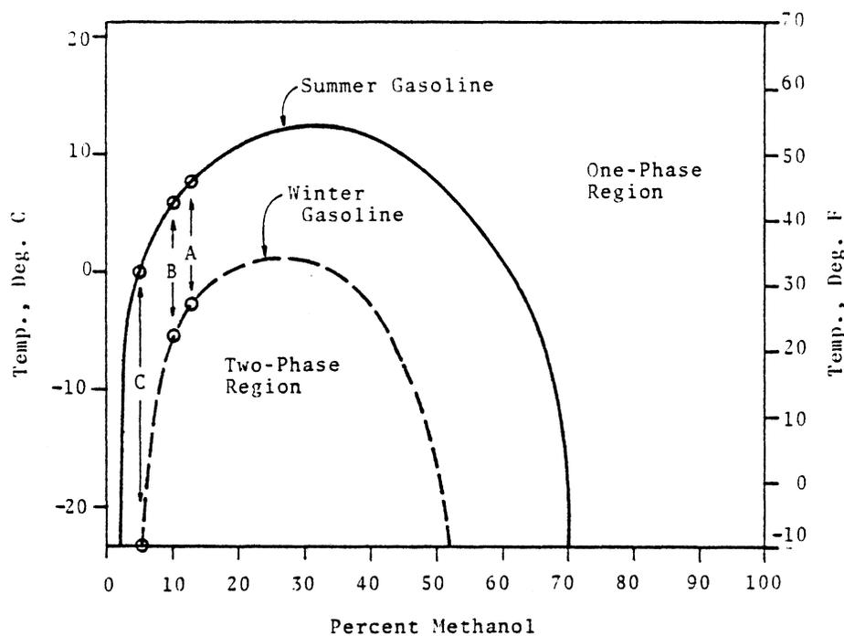
Figure 5. Separation of methanol in gasoline as a function of temperature. [After Reed et al.(9)]
