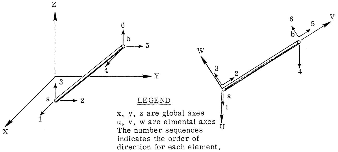
Figure A-1. Global and element axes for space truss element.
