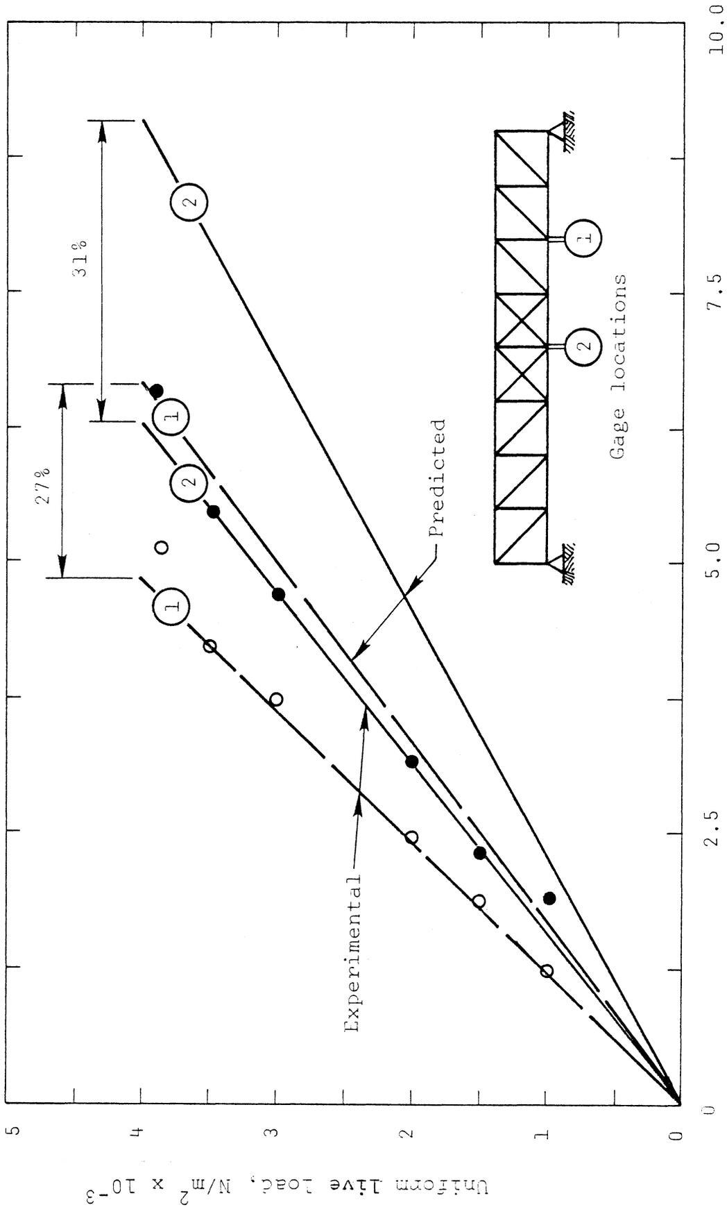
Figure 7. Comparison of theoretical and experimental deflections for live load test of girder.  $25.4 \text{ mm} = 1 \text{ inch}$ ;  $47.8 \text{ N/m}^2 = 1 \text{ psf}$ .
