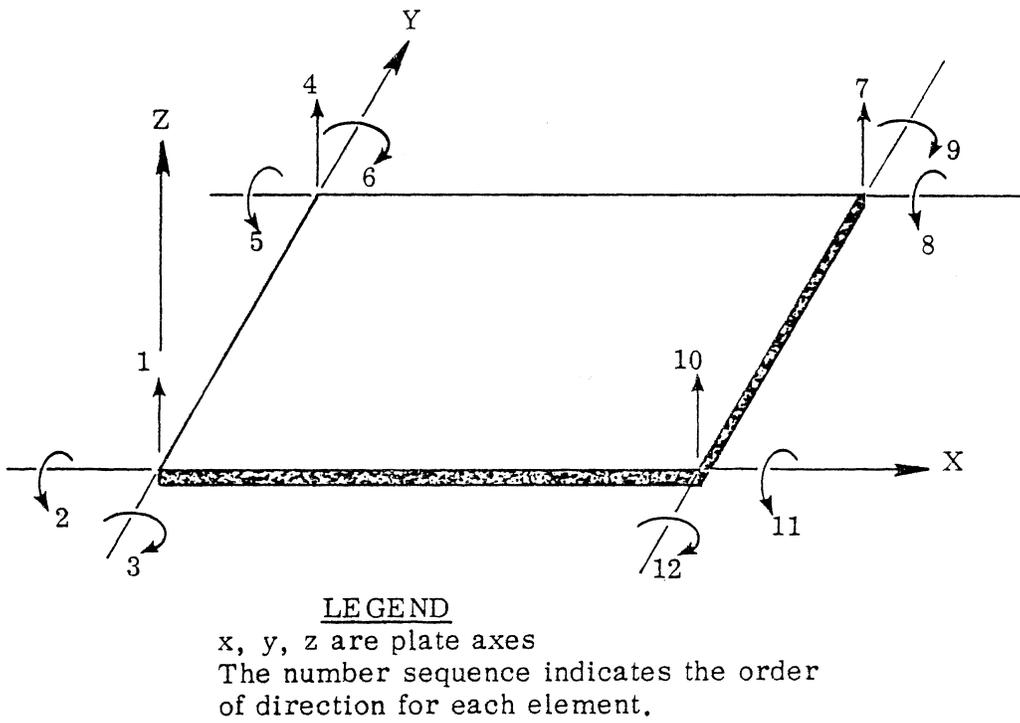
Figure A-2. Rectangular plate bending element.
