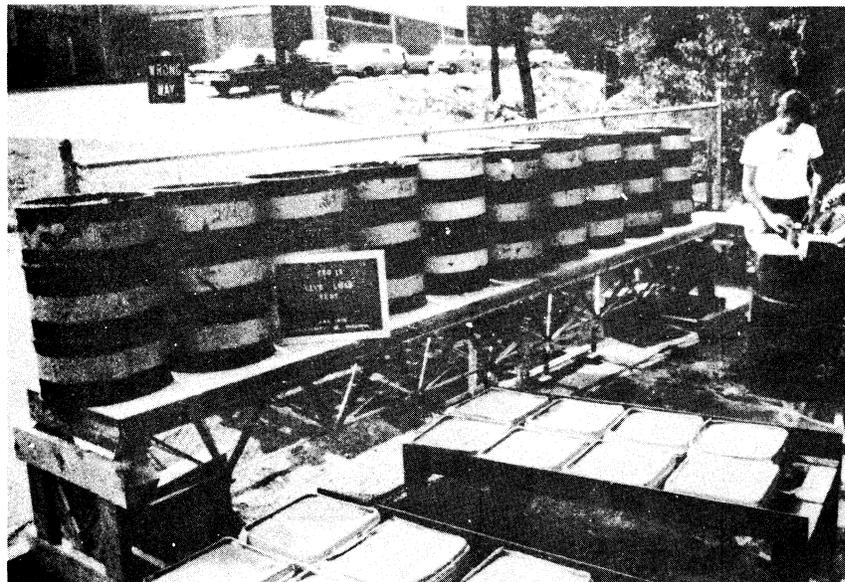
Figure 6. Live load test with water-filled barrels to a maximum of  $3680.6 \text{ N/m}^2$  (77 psf).
