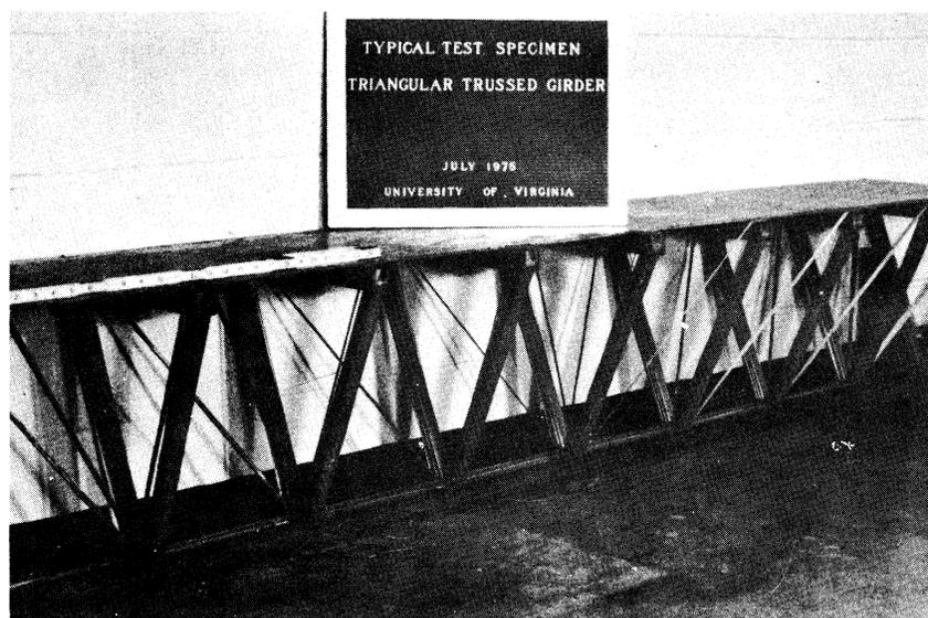
Figure 1. Typical test specimen of a triangular trussed girder showing principal features.
