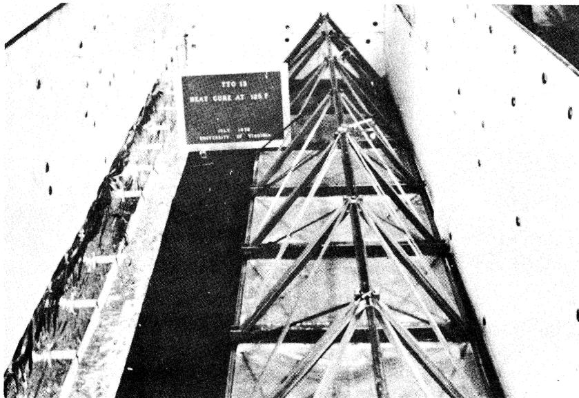
Figure 4. Completed girder in oven for postcuring resin at  $54.4^{\circ}\text{C}$  ( $130^{\circ}\text{F}$ ).
