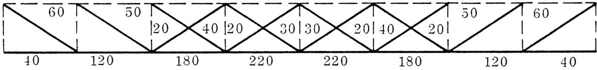
Winding paths and total tension strands for TTG-WC. (Dashed lines are stiffeners and plate.)
