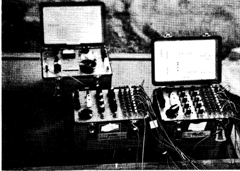
Figure 14. Two portable digital strain indicators and switch and balance unit.
