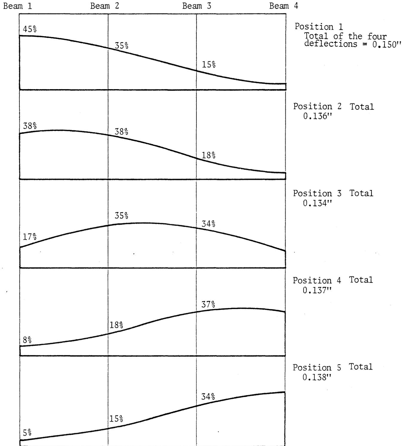
Figure 20. Percentage of live load distributed to concrete girders on basis of deflections.
