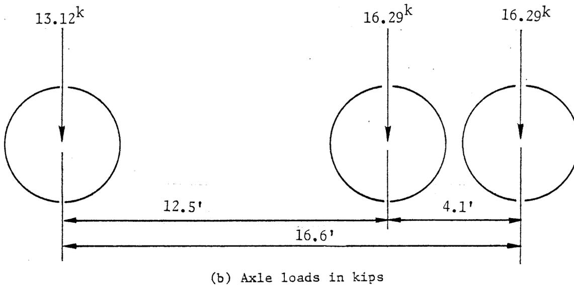
Figure 15. Axle dimensions and axle loads of the test vehicle.
