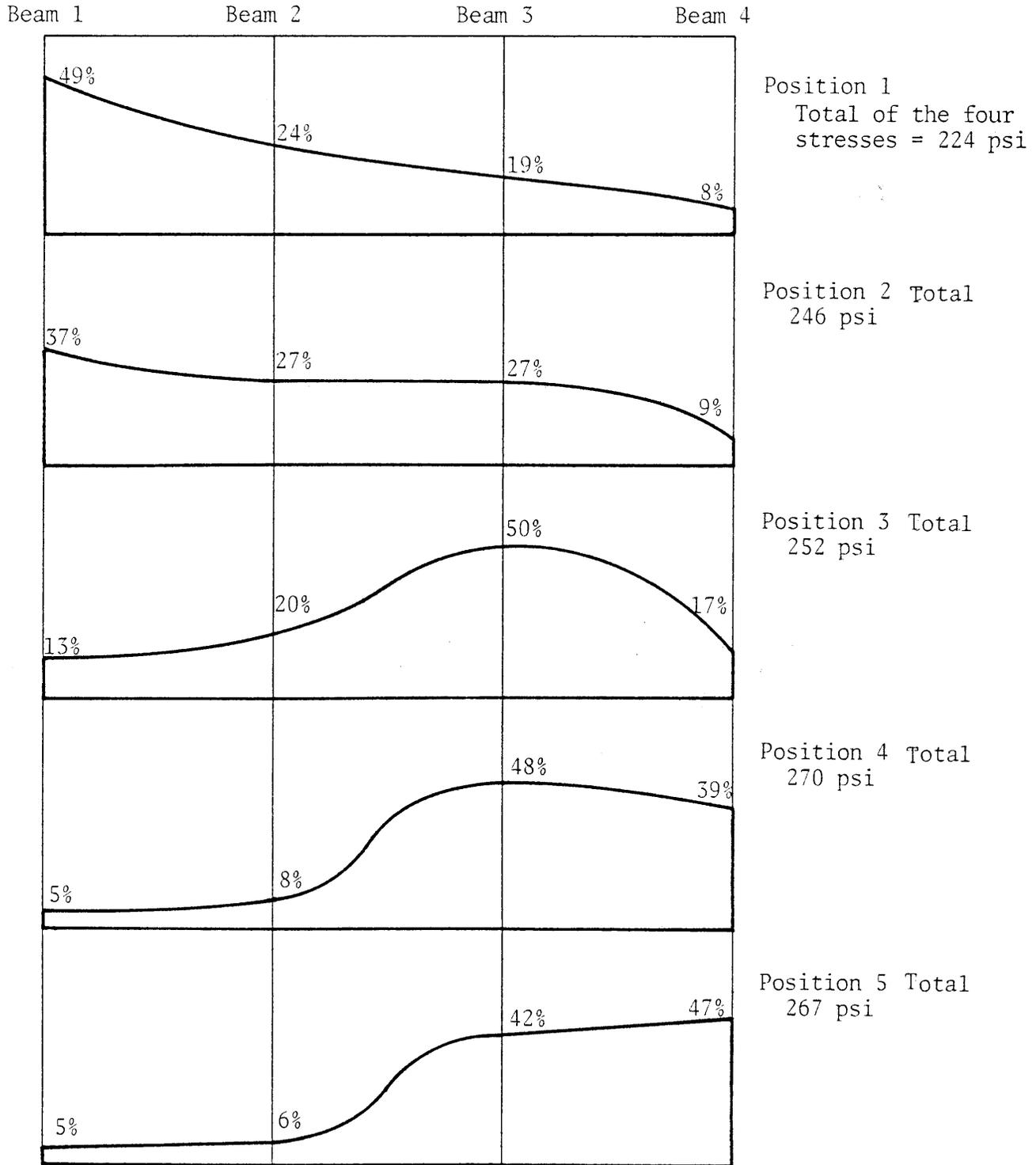
Figure 19. Percentage of live load distributed to concrete girders on basis of stresses.
