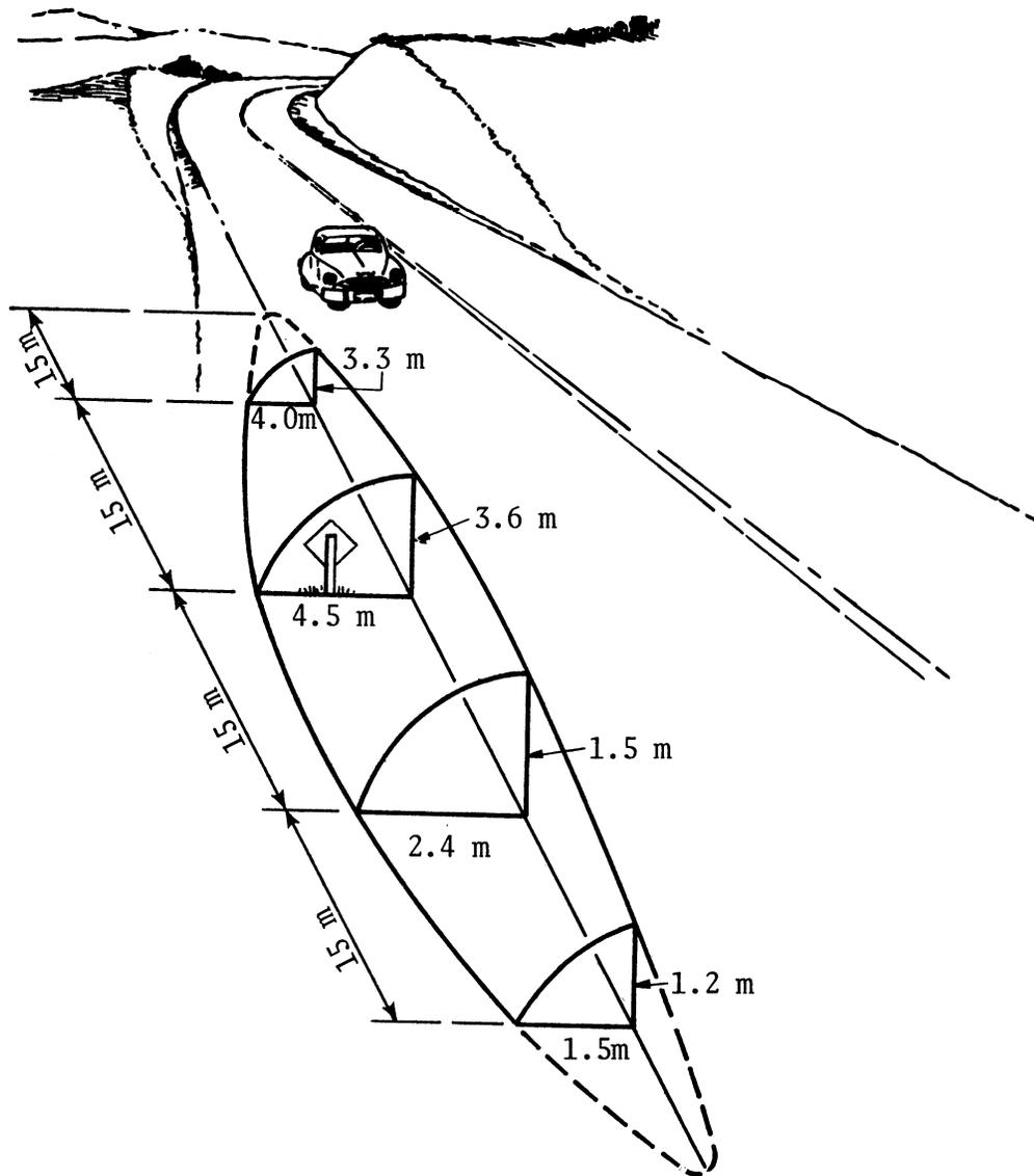
Figure 2. Keg of good legibility of 0.6 m x 0.6 m (1 m = 3.3 ft.) diagrammatic reflective sign under low beam headlights.
