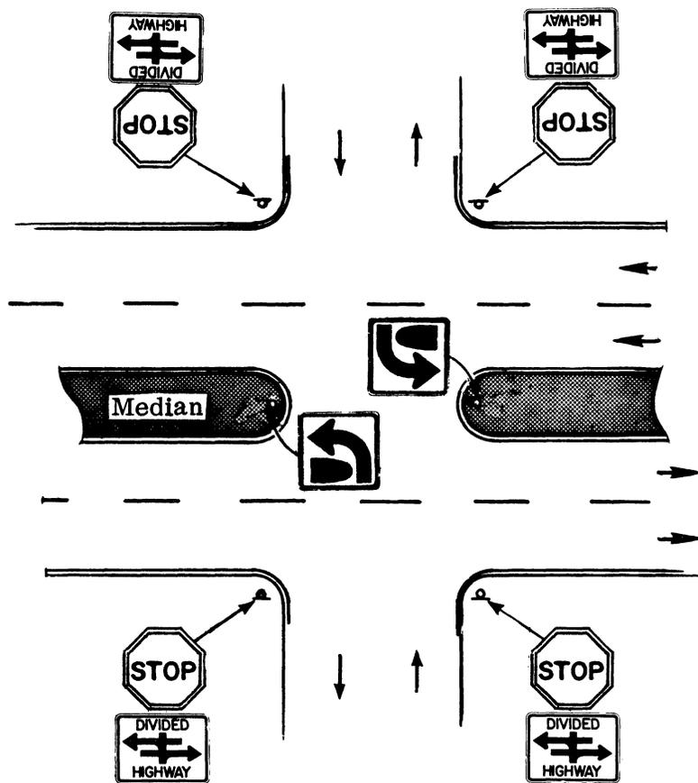
Figure 10. Recommended traffic signs for discouraging wrong-way entry.
