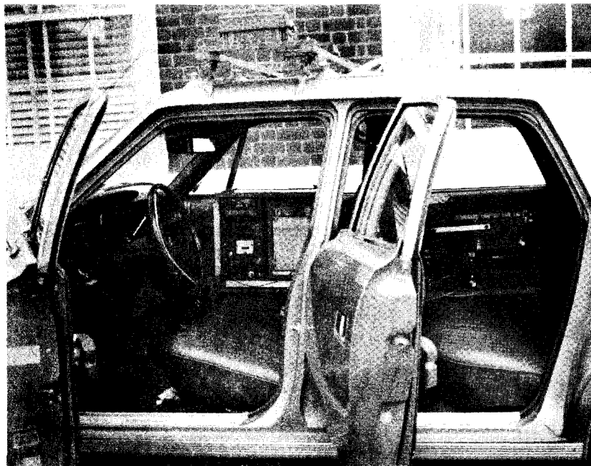
Figure 5. Illumination recording equipment installed in a vehicle.
