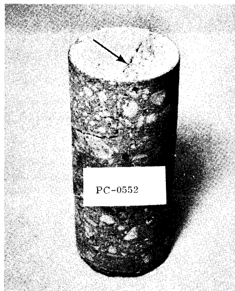
Figure 11. Appearance at pavement surface of distress between patch and existing concrete. Note: Core dimensions are 4 in. x 9 in. (100 mm x 230 mm).
