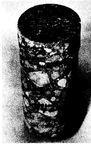
Figure 9. Large void in zone between patch and underlying old concrete due to inadequate consolidation. Note: Core dimensions are 4 in. x 9 in. (100 mm x 230 mm).
