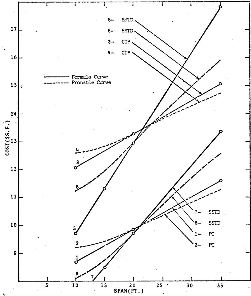
Figure 31. Total superstructure costs compared for the three types of construction for span lengths between 10' and 35'.
