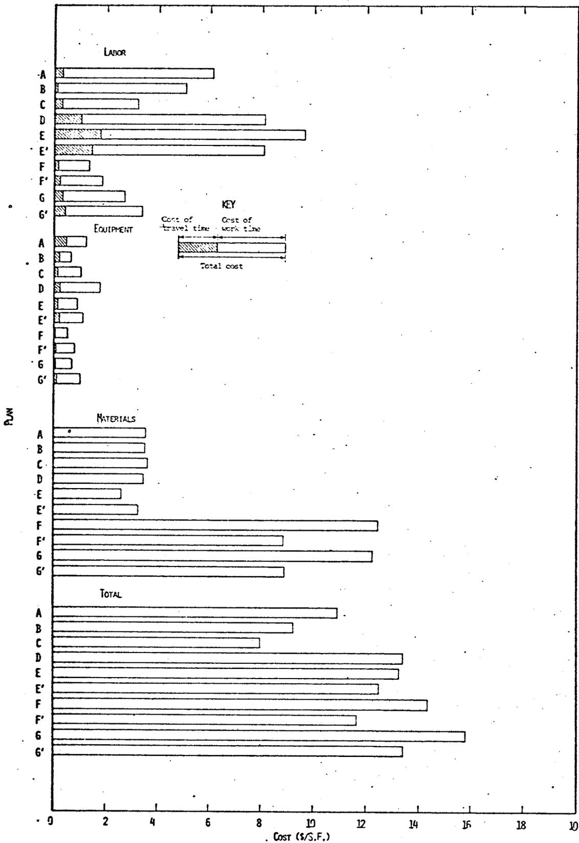
Figure 26. Comparison of labor, equipment, material, and total costs per square foot for 10 plans.
