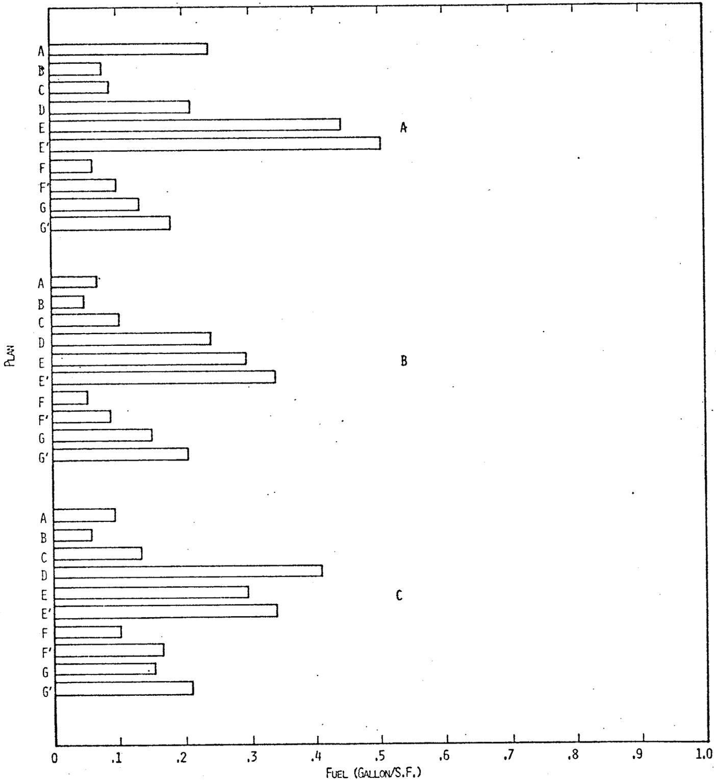
Figure 28. Plans compared with regard to fuel consumed by construction equipment in traveling between bridge site and district or residency with actual values (A), uniform travel distance (B), and uniform travel distance and work crew size (C).
