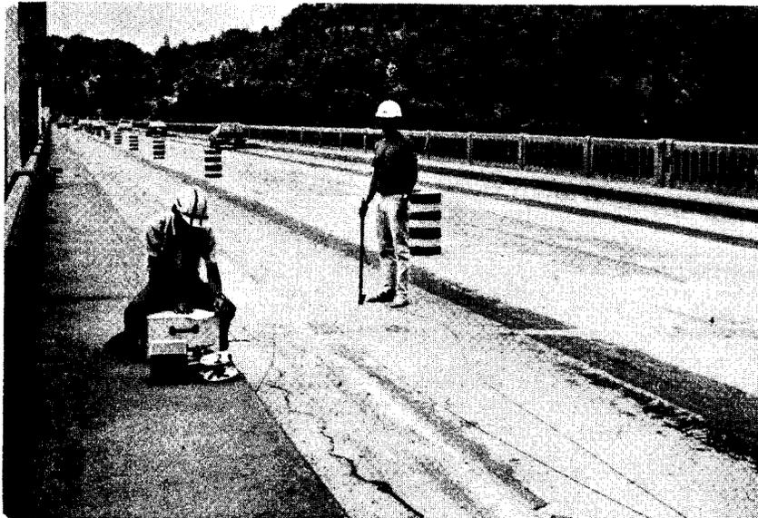
Figure 12. Corrosion potential measurements in progress.
