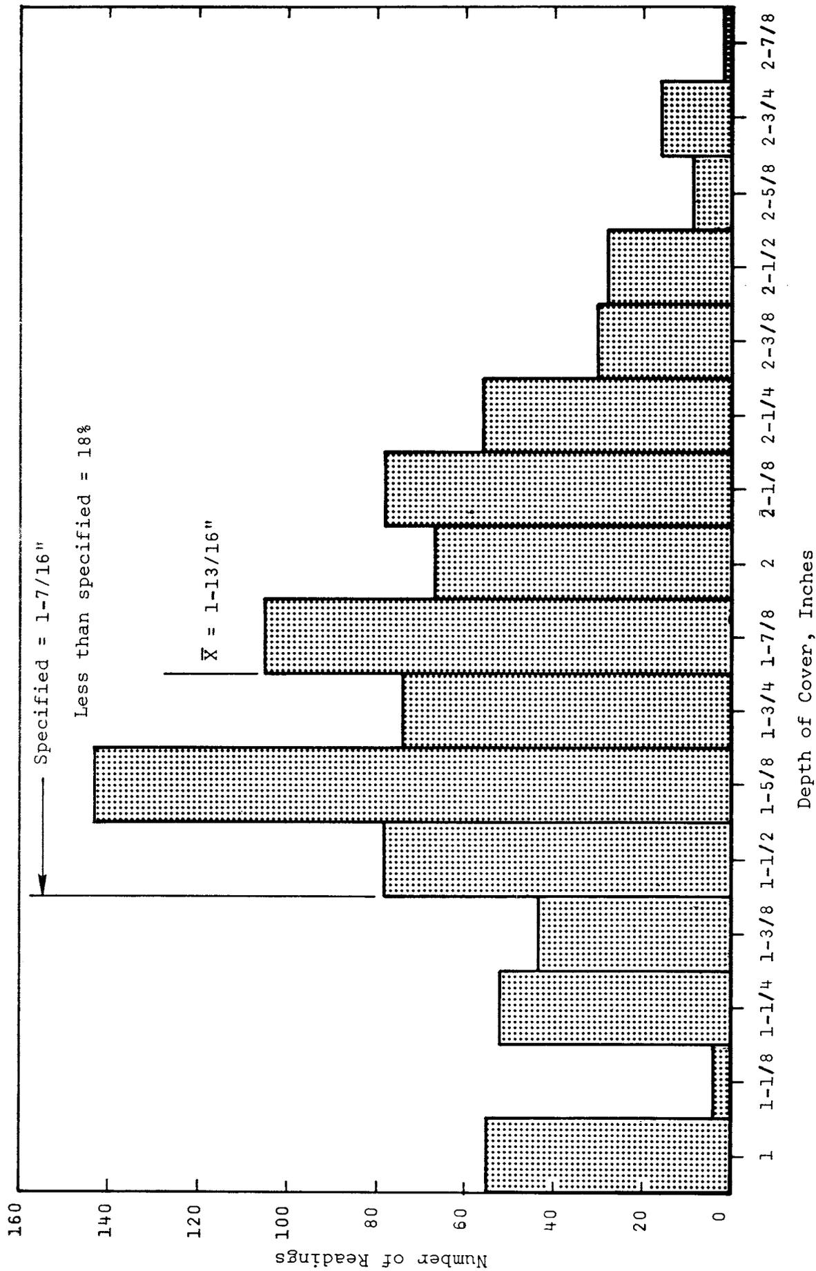
Figure 10. Distribution of cover depths - South Fork structure.
