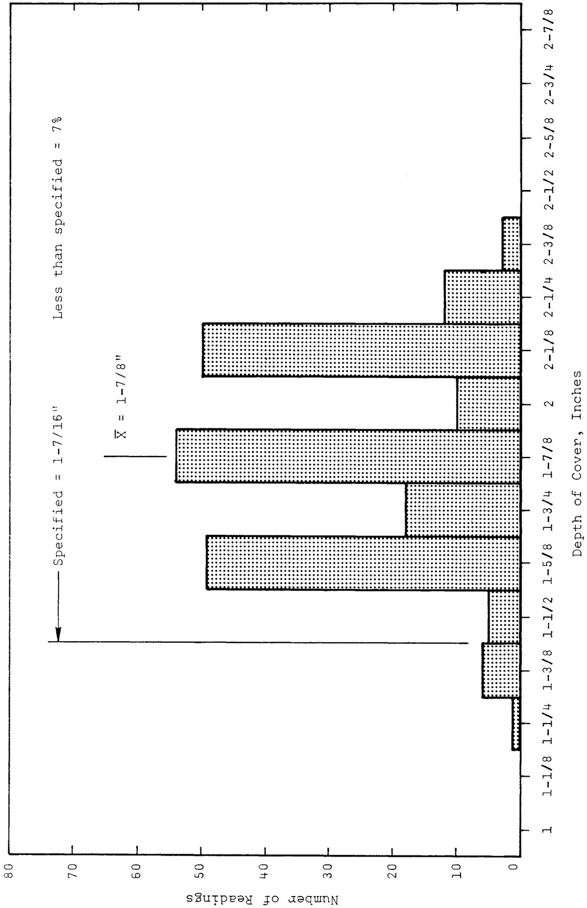
Figure 11. Distribution of cover depths — North Fork structure.
