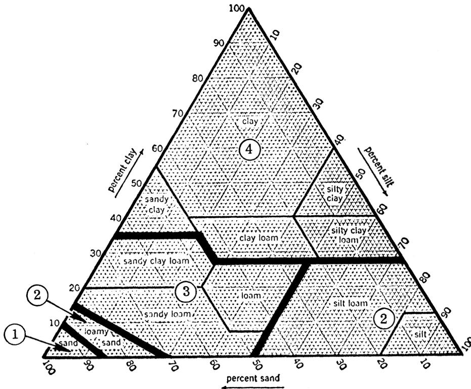
Figure 4. Chart for estimating structure index of soil by using percentages of clay (below 0.002 mm), silt (0.002 to 0.05 mm), and sand (0.05 to 2.0 mm).
