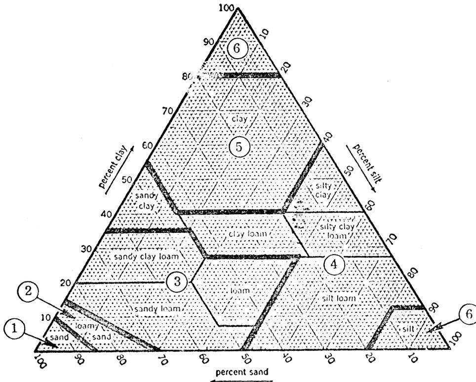
Figure 5. Chart for estimating permeability class of soil by using percentages of clay (below 0.002 mm), silt (0.002 to 0.05 mm), and sand (0.05 to 2.0 mm).
