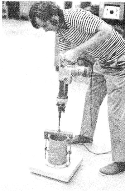
Figure 1. Compaction of specimen with vibratory rammer.
