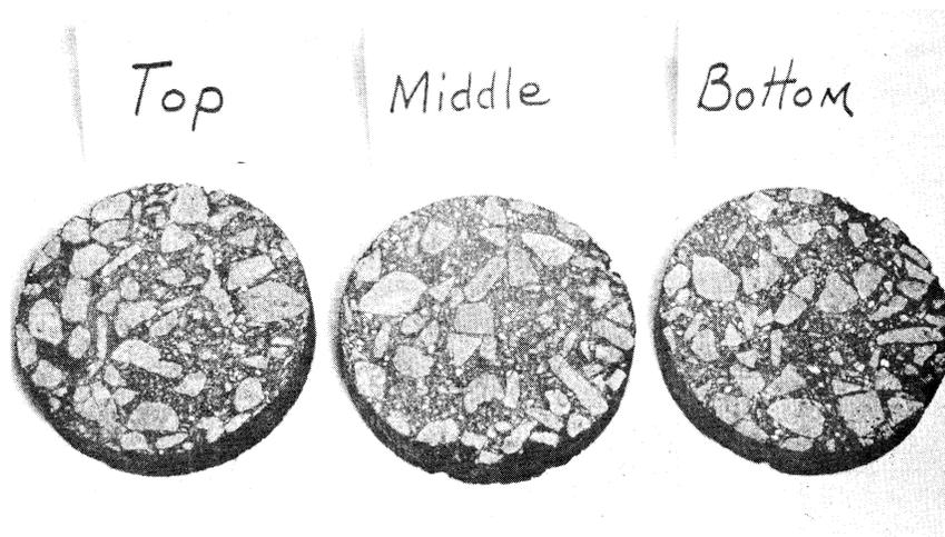
Figure 4. Sawed sections of specimen compacted with drop hammer.
