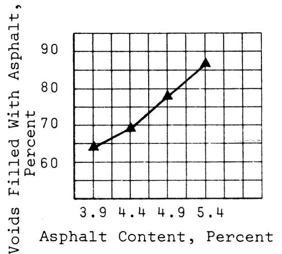
Figure 5. Asphalt content vs. #1 mix properties.
