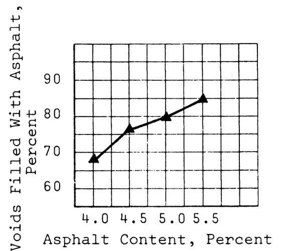
Figure 7. Asphalt content vs. #3 mix properties.
