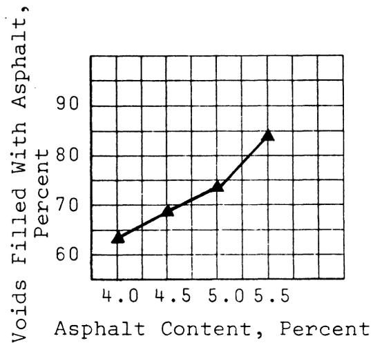
Figure 9. Asphalt content vs. #5 mix properties.
