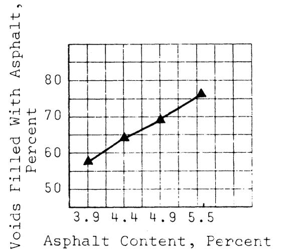
Figure 6. Asphalt content vs. #2 mix properties.
