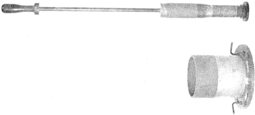
Figure 2. Drop hammer and mold assembly.
