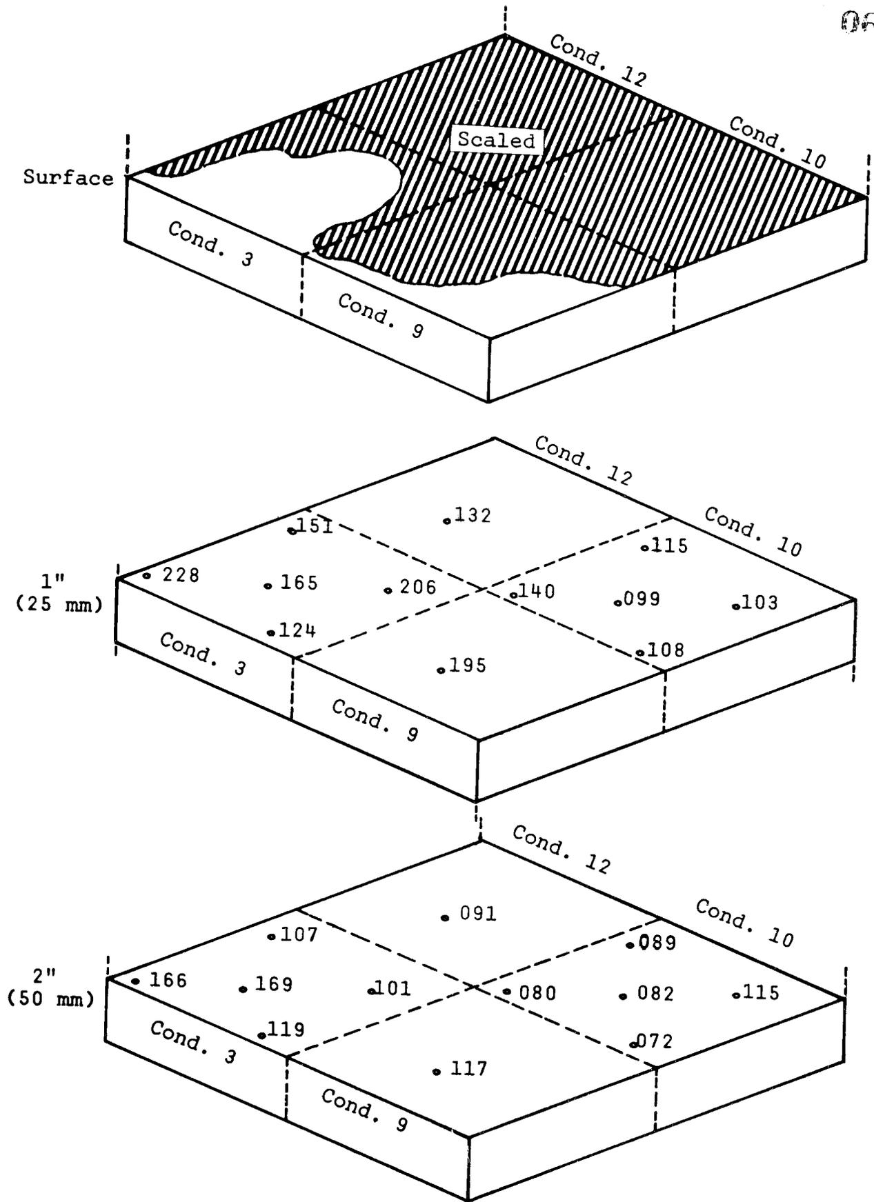
Figure 5. Location of samples and results of chloride analyses for slab 2N (Non-air entrained).
