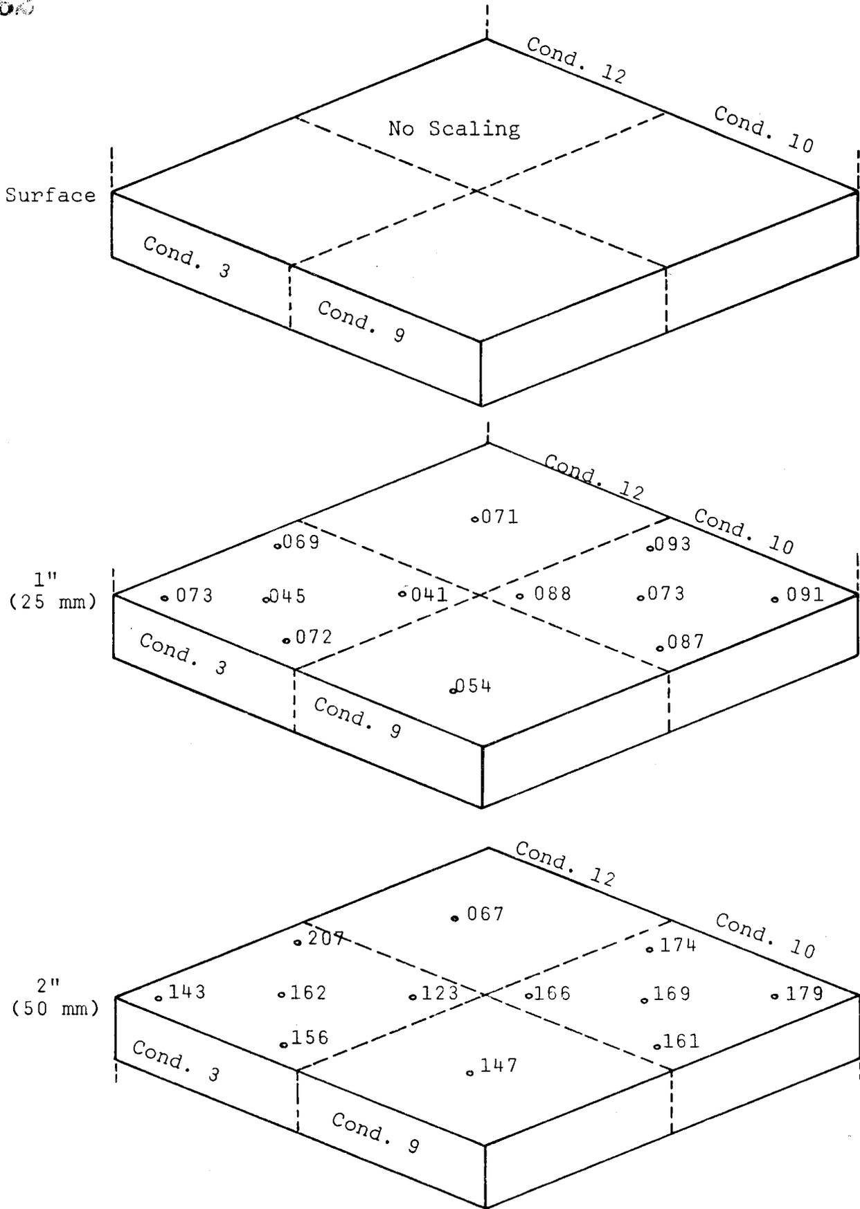
Figure 6. Location of samples and results of chloride analyses for slab 2A (Air entrained).
