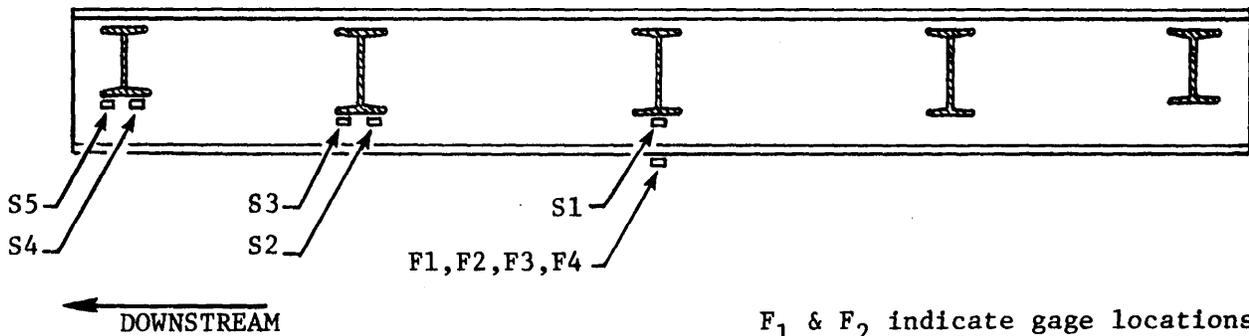
$F_1$  &  $F_2$  indicate gage locations on floorbeam at  $L_1$
