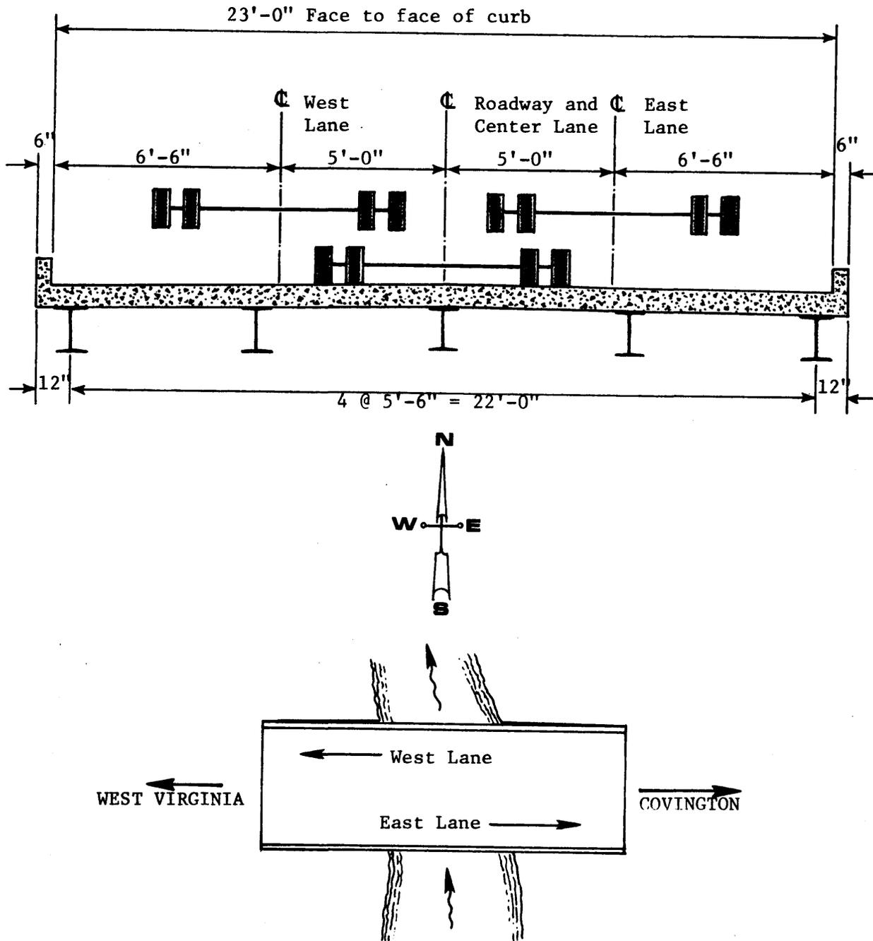
Figure 11. Lane positions and bridge orientation.
