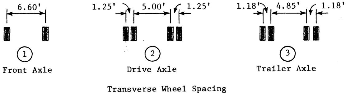
Figure 10. Simulated HS loading used in test.
