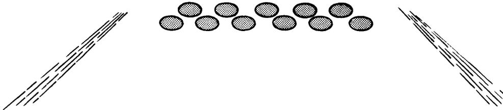
Figure 2. Arrangement of cutting heads for scabbler.
