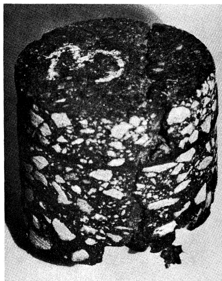
Figure 3. Core through new overlay (top), Petromat, and old overlay. Route 460 project.
