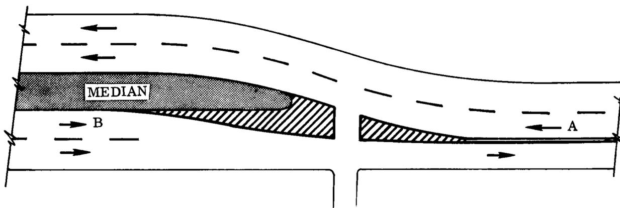
Figure 21. Stripping and its visibility at night is essential for preventing wrong-way entries from A to B at night.
