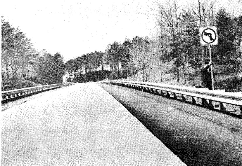
Figure 2. Day photograph of 8 ft. (2.4 m) high sign at 50 ft. (15 m) from the driver and 10 ft. (3 m) lateral distance.
