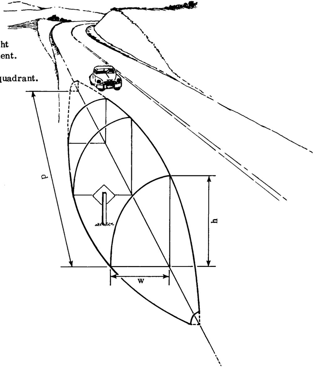
Figure 4. Keg of good legibility of 2 ft. x 2 ft. diagrammatic reflective sign under low beam headlights.
