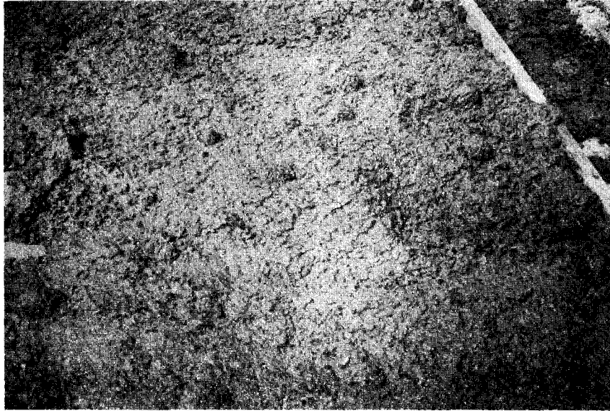
(a) Numerous wire fiber balls in the trial installation mix.
