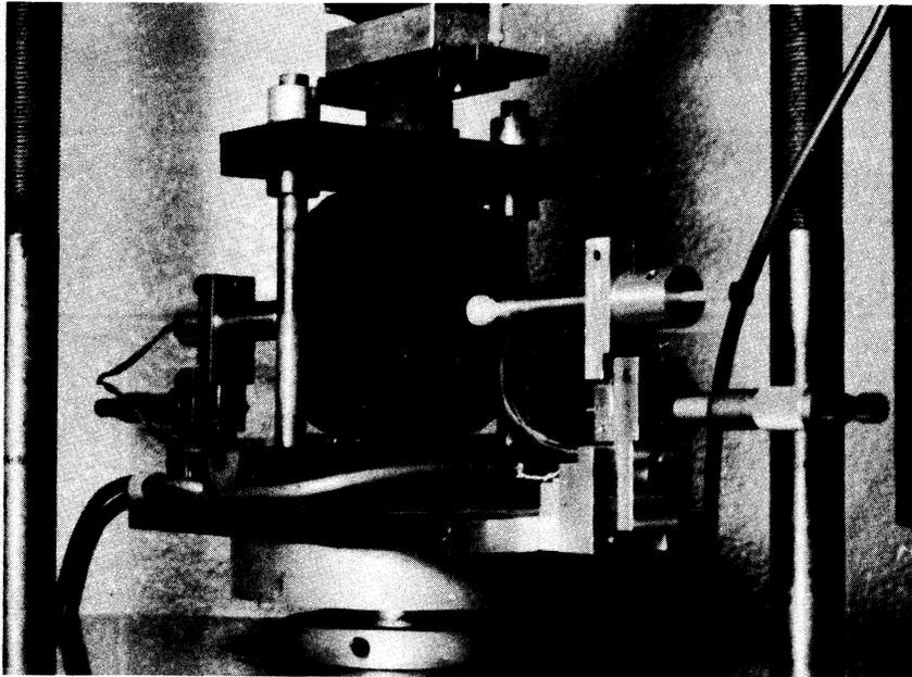
Figure 2. Indirect Tensile Test.
