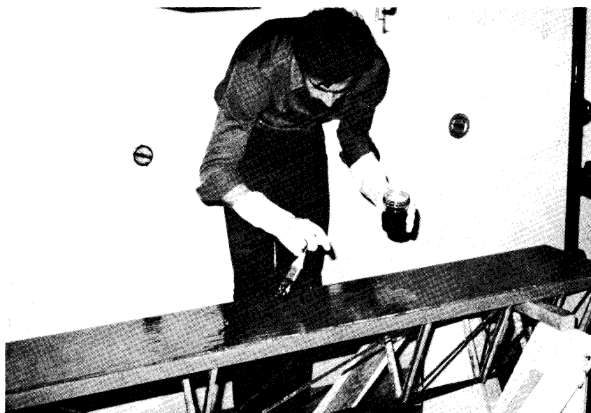
Figure 6. Application of resin binder for top cover plate on TTG-3.
