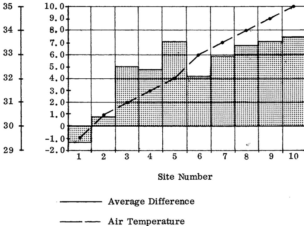
Figure 6. Dependence of instrumentation drift with temperature.
