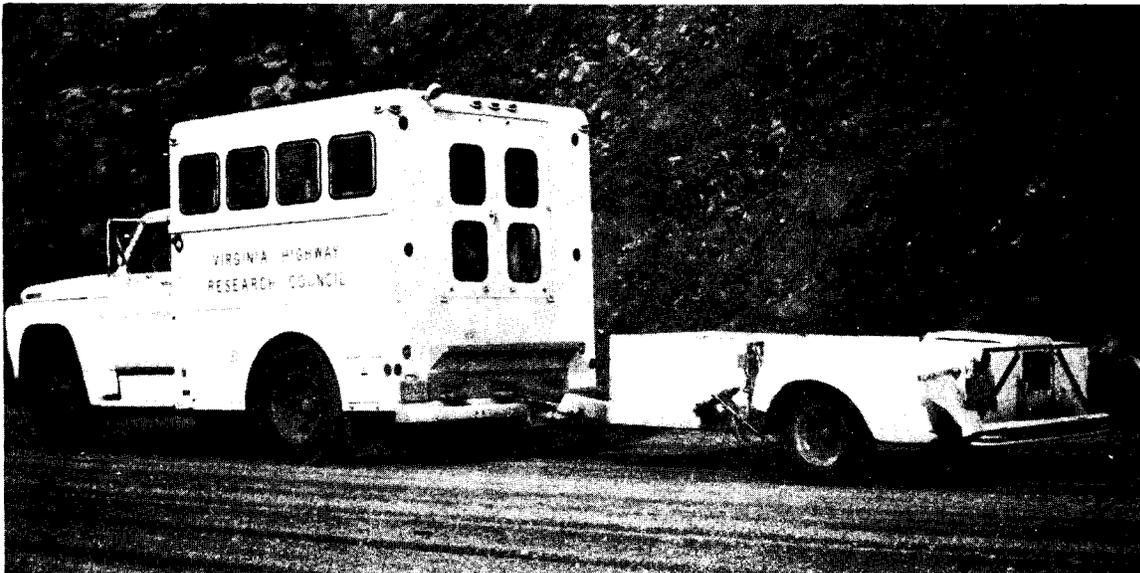
Figure 1. The VHRC, Model-2, skid-resistance measurement vehicle.
