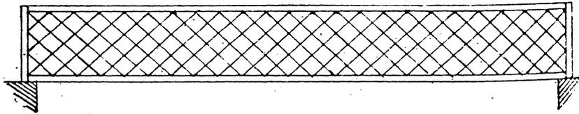
Figure 3. Ithiel Town's all timber "Lattice truss", patented in 1820. (From A Span of Bridges, H. J. Hopkins, p. 118.)
