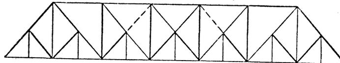
Figure 13. Baltimore/Petit truss, a Pratt truss having subdivided panels. (From Bridge Engineering, James A. L. Waddell, p. 469.)
