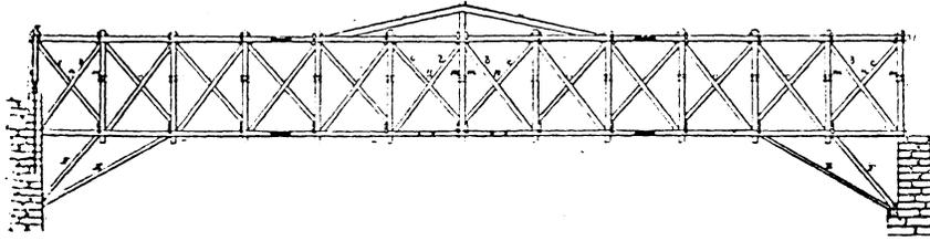
Figure 4. Stephen H. Long's panel truss timber bridge patented in 1830. (From American Building, Carl Condit, illus. 16.)
