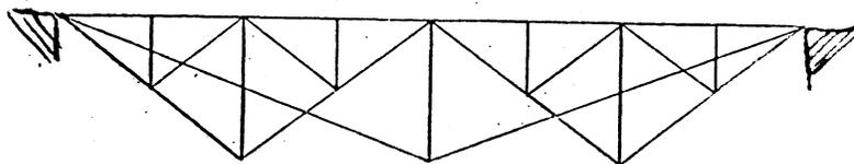
Figure 10. Albert Fink's suspended truss patented in 1854. (From Bridge Engineering, James A. L. Waddell, p. 473.)
