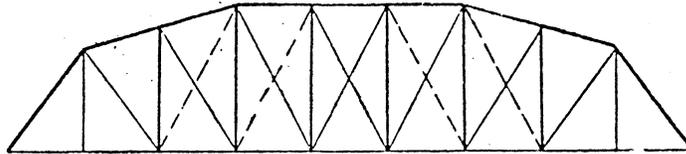
Figure 12. Camelback truss, again a Pratt truss configuration; however, here the polygonal top chord changes slope at alternating panel points. (From Bridge Engineering, James A. L. Waddell, p. 478.)
