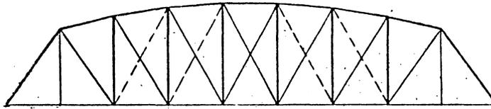
Figure 11. Parker truss, really a Pratt truss having a polygonal top chord whose slope changes at each panel point. (From Bridge Engineering, James A. L. Waddell, p. 469.)
