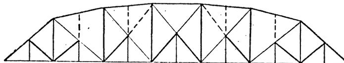
Figure 14. Pennsylvania truss, combination of Pratt, Camelback and Baltimore features. (From Bridge Engineering, James A. L. Waddell, p. 470.)
