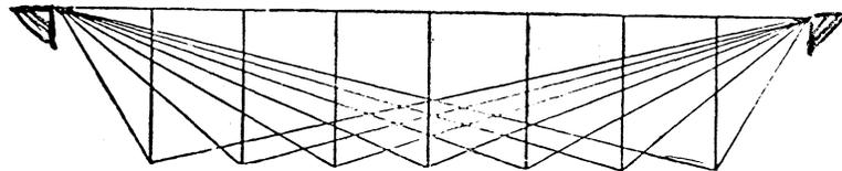
Figure 9. Wendel Bollman's suspended truss patented in 1852. (From Bridge Engineering, James A. L. Waddell, p. 473.)
