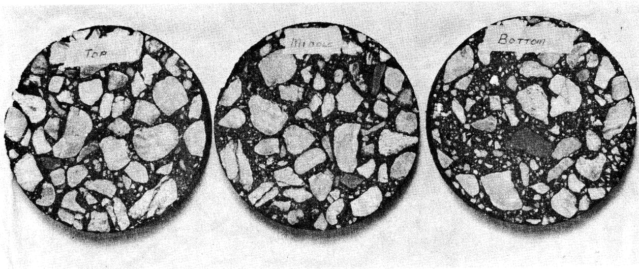
Figure 2. A lab specimen sawed into three sections for obtaining densities.
