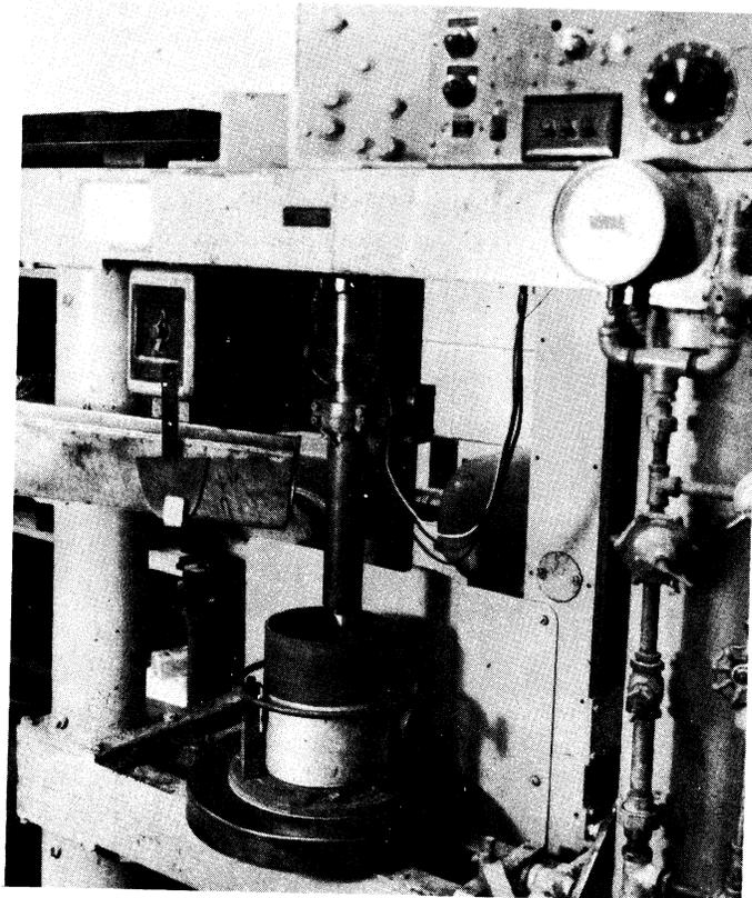
Figure 1. California kneading compactor, 6" mold, and accessories used to make specimens.
