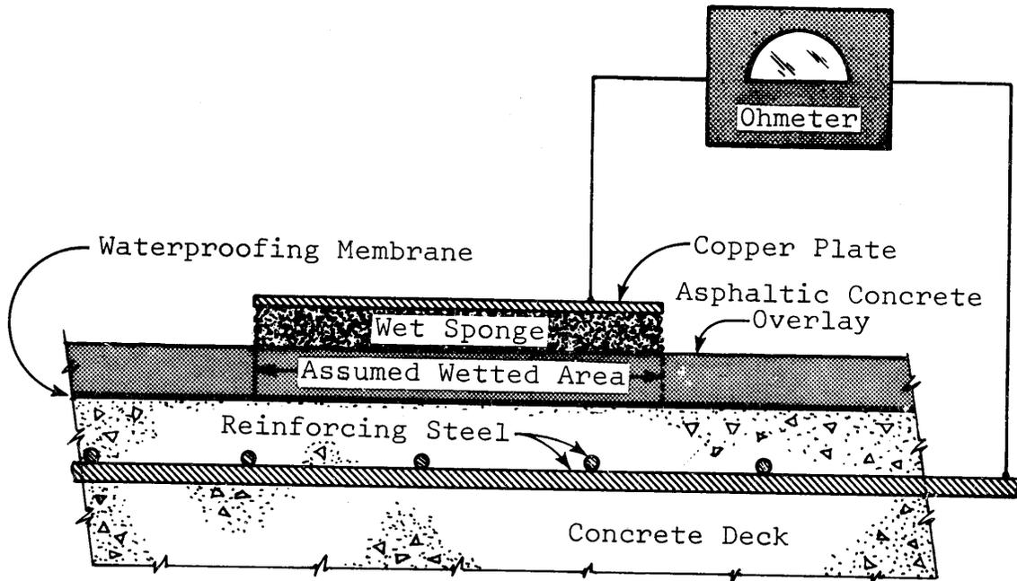
Figure 1. Assumed circuit for the electrical resistivity test.
