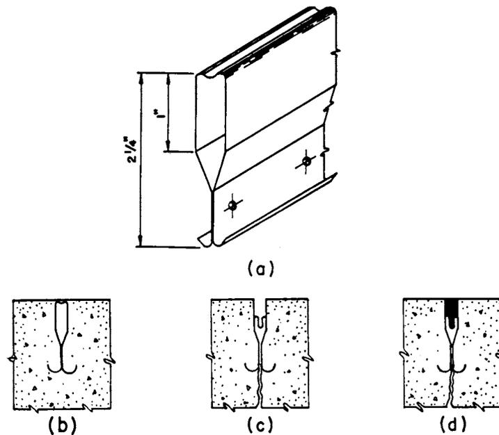
Figure 1. Tabular metal joint insert: (a) cross section of 2 1/4" insert, (b) as installed, (c) after crimping, and (d) after sealing. Basic conversion unit: 1" = 25.4 mm.
