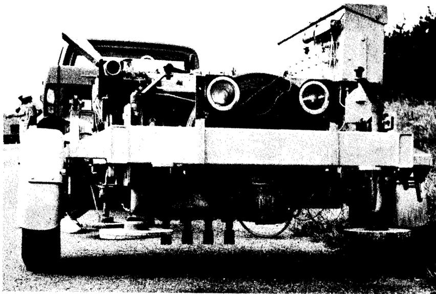
Figure 5. Rear view of small hole cutting machine with cutting heads visible.
