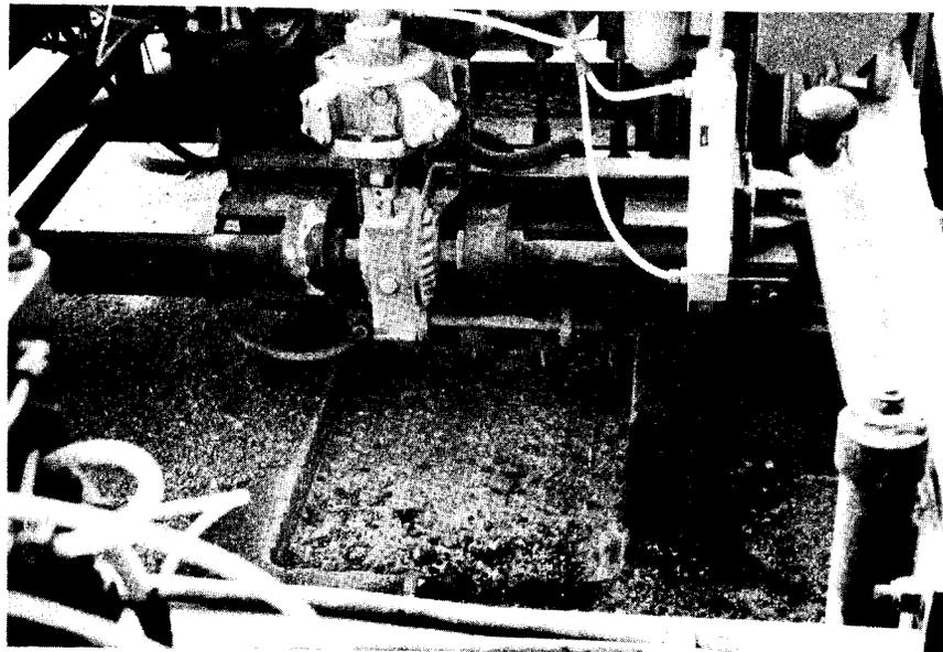
Figure 6. Small machine in hole cutting operation.
