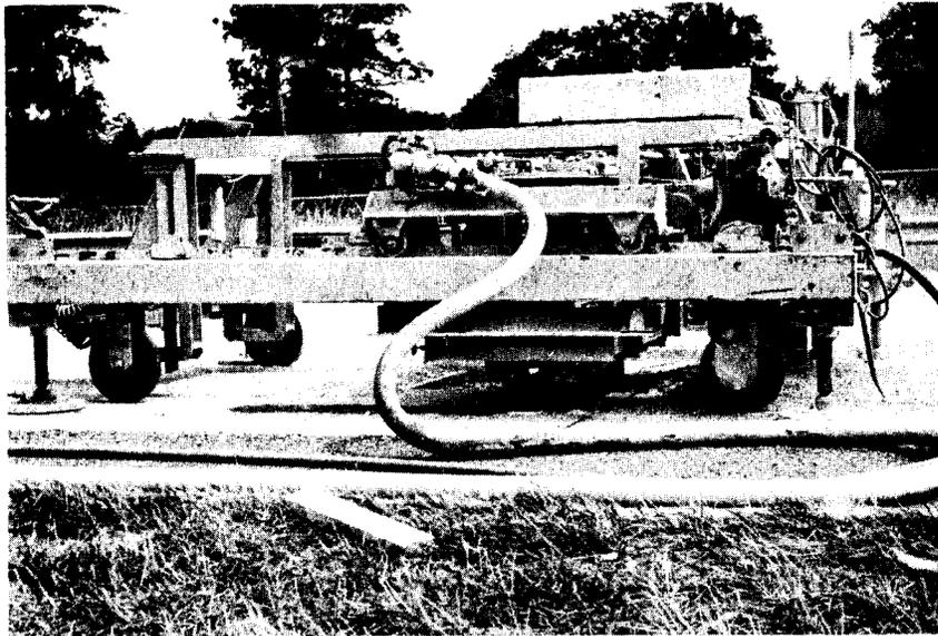
Figure 4. General purpose concrete repair machine in a hole cutting operation.
