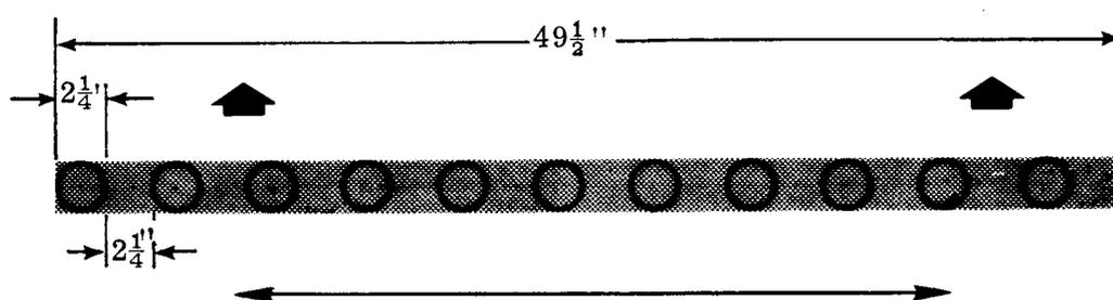
Figure 3. Configuration of cutting heads of the general purpose concrete repair machine. (Two-headed arrow indicates that the heads move to right and left on a transverse carriage to cut area in between.)
