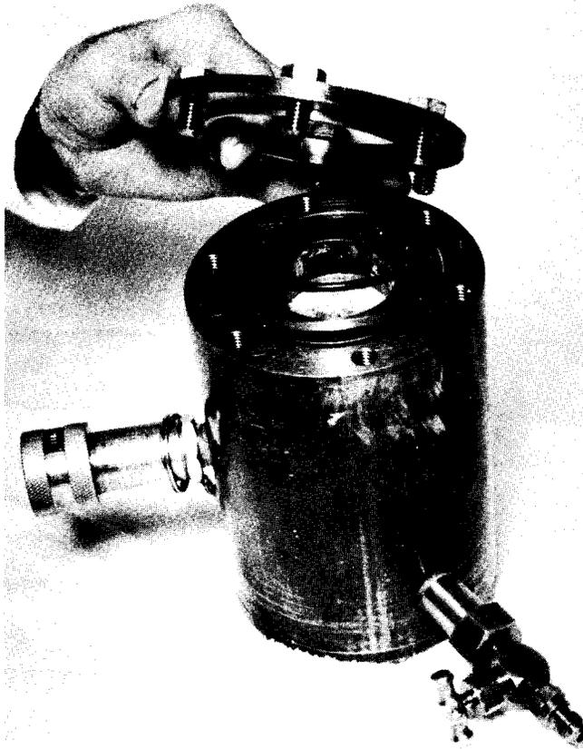
Figure 5. Concrete cylinder in test chamber.
