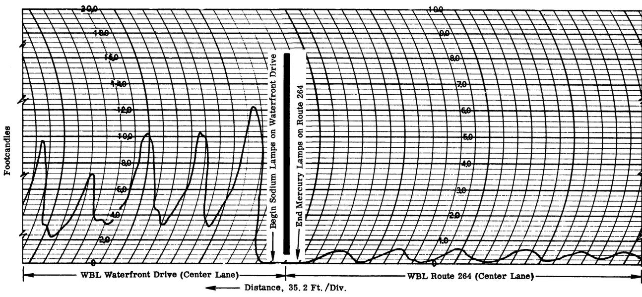
Figure 4. Contrasting illumination levels in the transition area between the mercury lighting on I-264 and the sodium lighting on Waterfront Drive. (Note the difference in the fc. scale factor for the sodium lights in the RHL as opposed to the center lane.)
