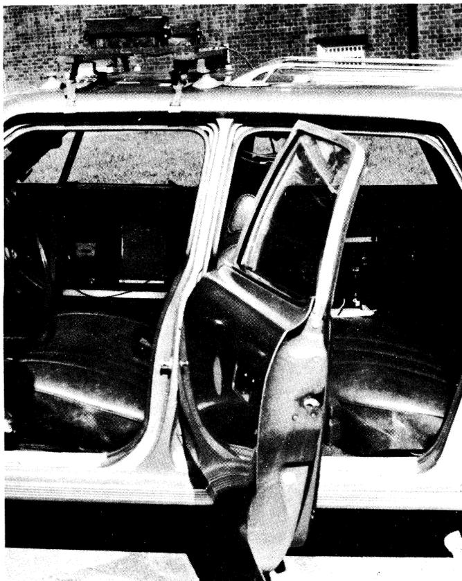
Figure 1. Mobile illumination recording instrumentation with photocells mounted on the roof of the vehicle.
