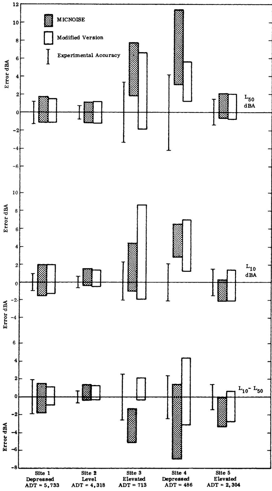
Figure 14. 68% confidence levels on errors (calculated minus measured) for MICNOISE and for the modified MICNOISE version.
