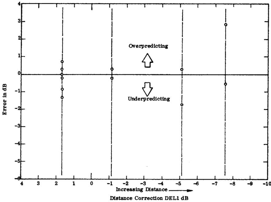
Figure 13. Errors in  $L_{50}$  (calculated minus measured) vs. distance correction  $DEL_1$  for near lane group, site 2.
