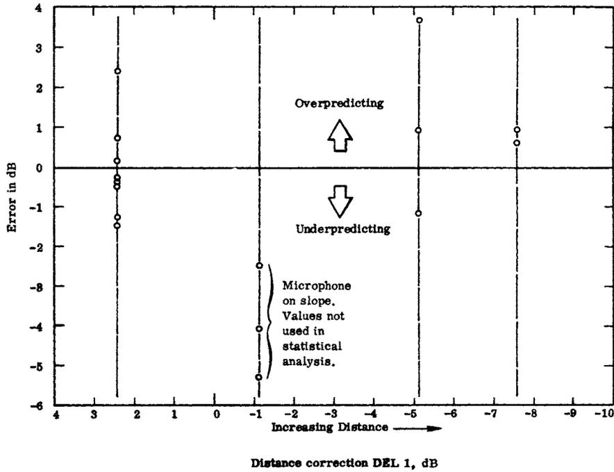
Figure 12. Errors in  $L_{50}$  (calculated minus measured) vs. distance correction  $DEL_1$  for near lane group, site 1.
