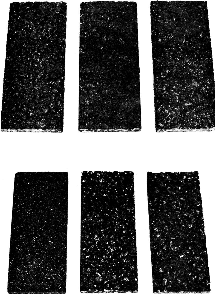
Figure 3. Test beams: top row — left to right — slag, granite, and limestone; bottom row — sprinkle test beams, left to right — aluminum oxide, calcined kaolin 3 inches x 4 inches, and calcined kaolin 1/2 inch x 1/8 inch.
