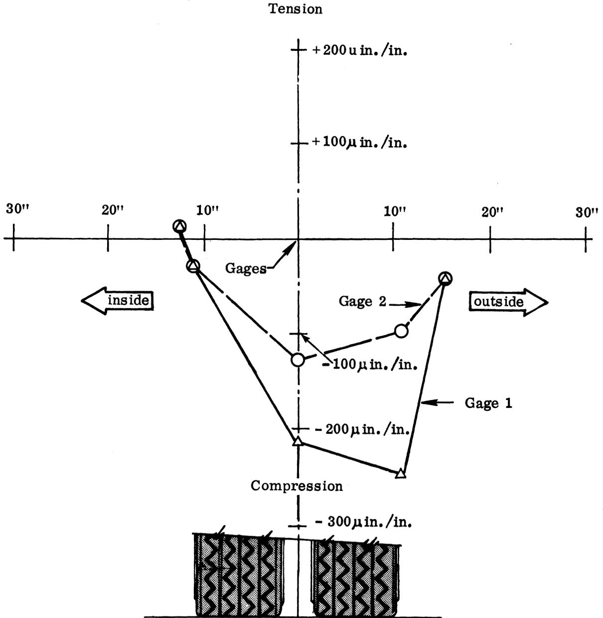
Figure A-2. Influence diagram for surface strain at  $\mathcal{C}$  of established wheelpath — Route 250.
