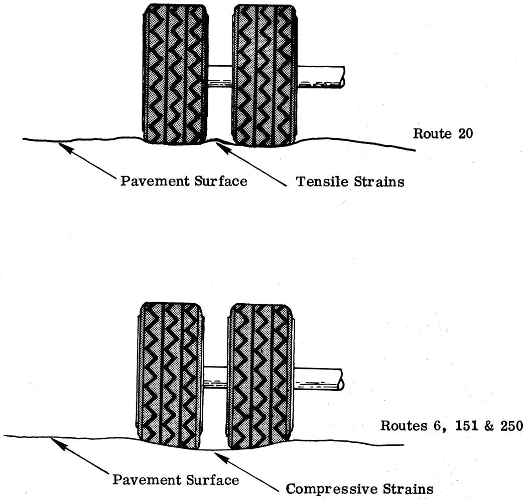
Figure 3. Possible strain and/or deflection configurations under dual wheel load.
