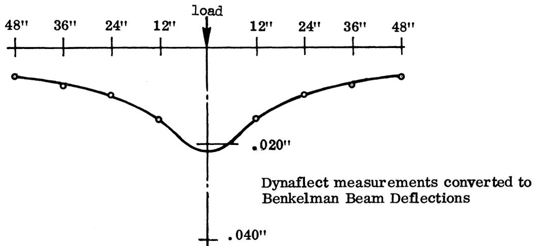
Figure A-3. Influence diagram for surface strain at  $\mathcal{L}$  of established wheelpath and dynaflect measurements — Route 151.
