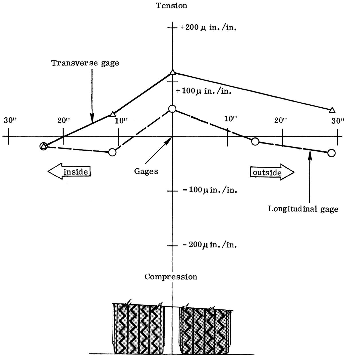
Figure A-1. Influence diagram for surface strain at C of established wheelpath - Route 20.
