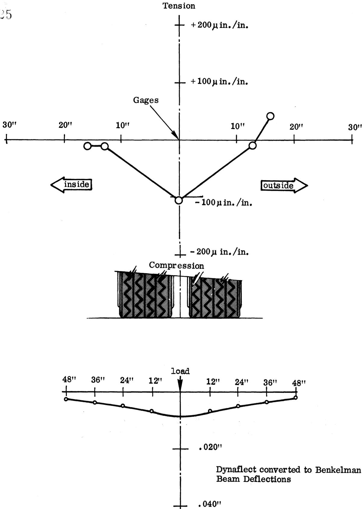
Figure A-4. Influence diagram for surface strain at  $\mathcal{C}$  of established wheelpath — and dynaflect measurements — Route 6.
