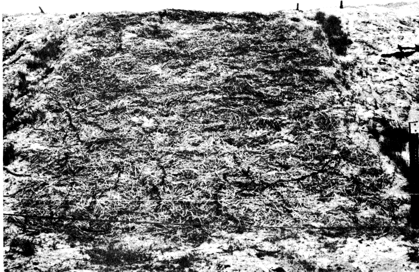
Plate 1. Conventional method used at all sites. 7 months — rating No. 1. This plot was treated at the rate of 2 tons of straw per acre tackied with 250 gallons of asphalt emulsion per acre.
