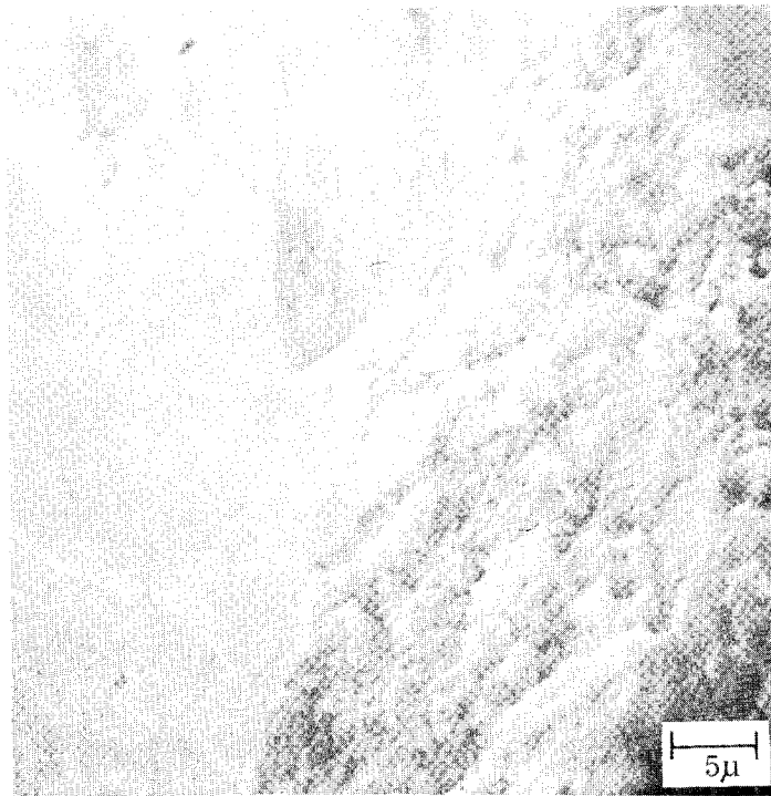
Figure 16. Microcline, 2,000 x, showing boundary between two types of surface morphologies shown in Figures 14 and 15. This micrograph represents views parallel to and perpendicular to cleavage.
