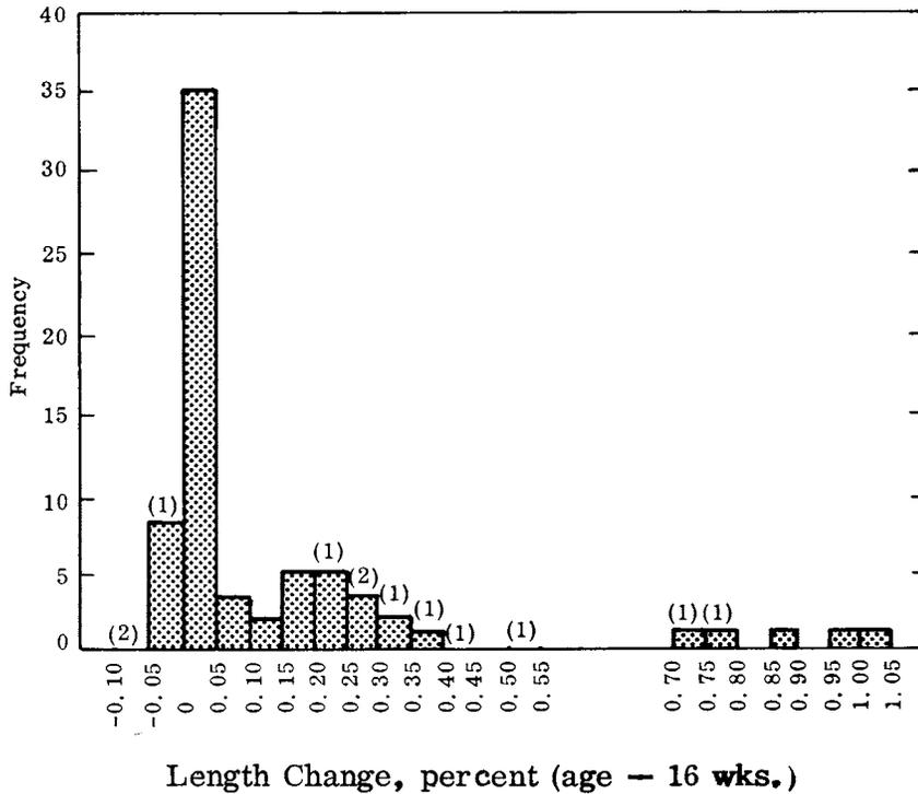
Figure 30. Distribution of length changes for prisms from Quarry 1. The bars represent results from the detailed survey (1964) and the numbers in parentheses indicate the number of samples exhibiting the indicated expansion in the preliminary statewide survey (1962).
