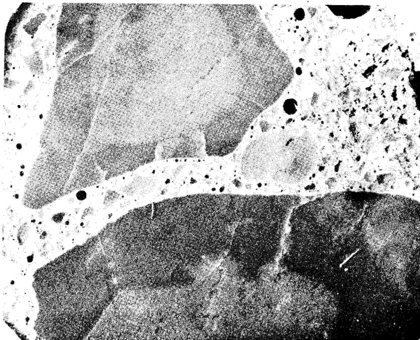
Figure 17. Aggregate 12-9 with low alkali cement. Expansion of concrete after 1 year equals 0.025%. Primary features are lack of cracking in mortar and pronounced rims on aggregates and cracks within rim areas. (7x)
