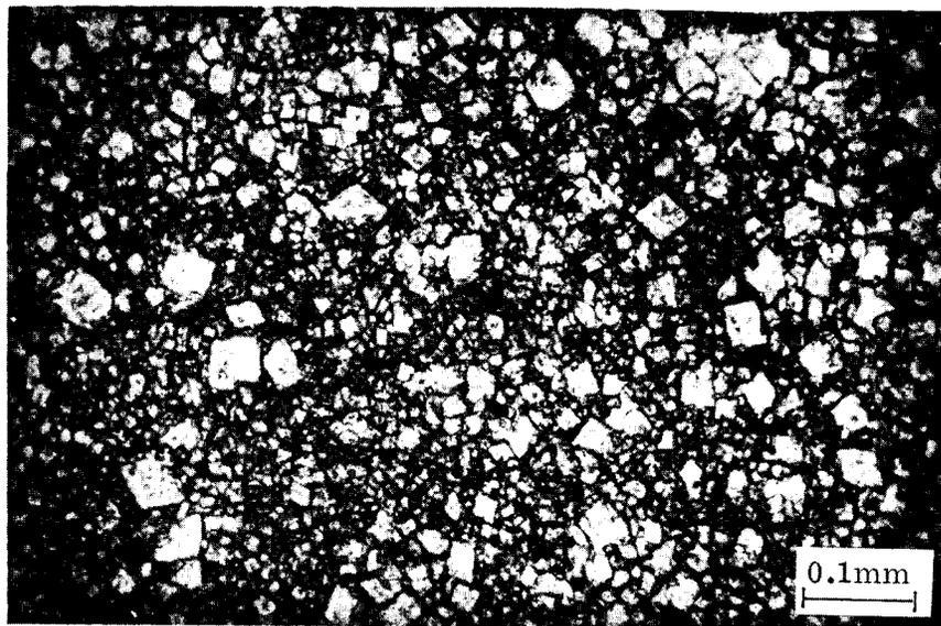
Figure 27. Texture of aggregate 23-9 representing material in concrete that showed expansion. (125x)
