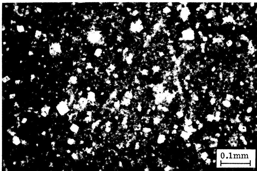
Figure 24. Usual texture of aggregate 12-1 showing areas of uniform microspar with a few isolated dolomite rhombs. (125x)
