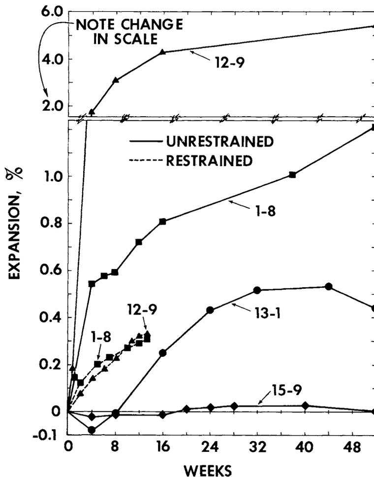
Figure 6. Length change of typical rock prisms.
