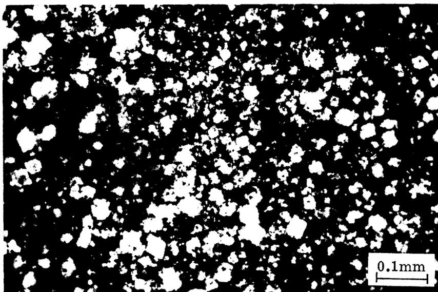
Figure 25. An area of well developed reactive texture in aggregate 12-1. (125x)
