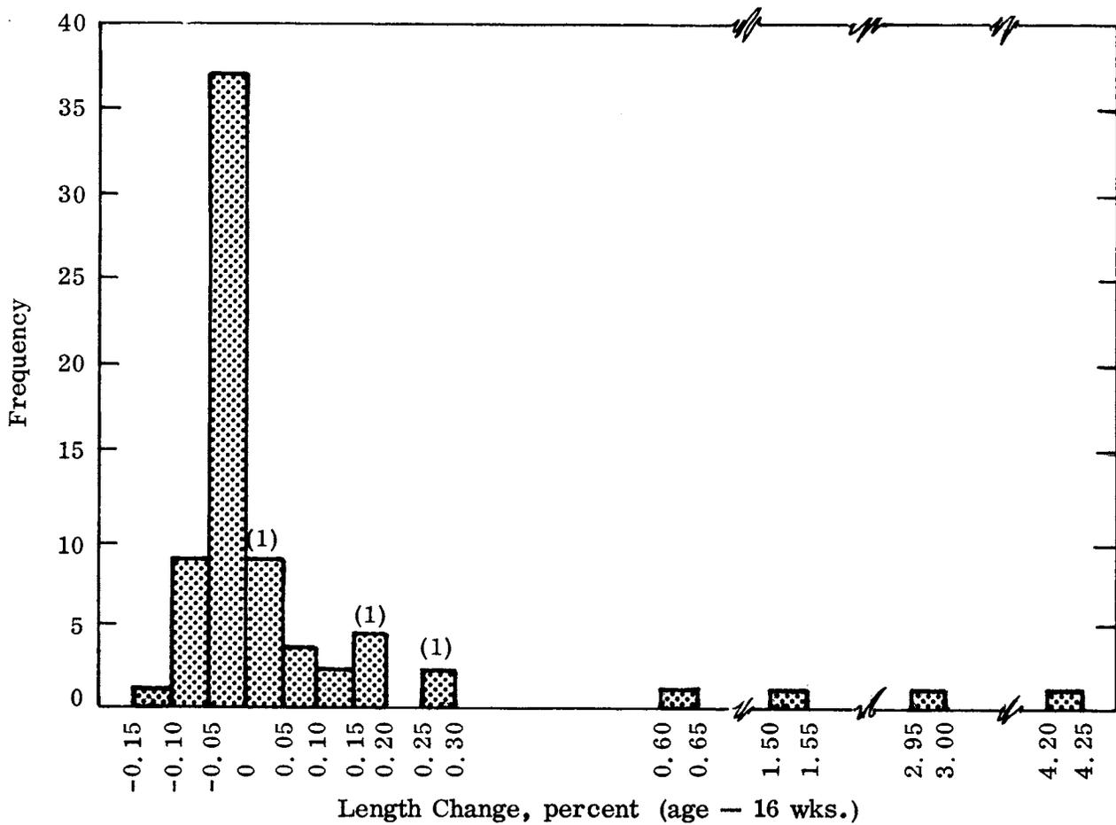
Figure 33. Distribution of length changes for prisms from Quarry 12 in the same form as shown in Figure 30.
