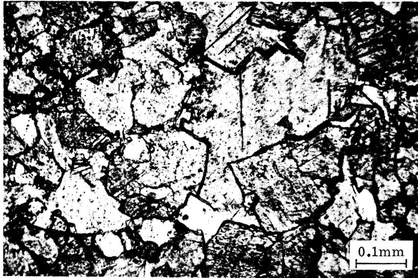
Figure 26. Texture of aggregate 23-9 representing material in prisms that did not expand. (125x)
