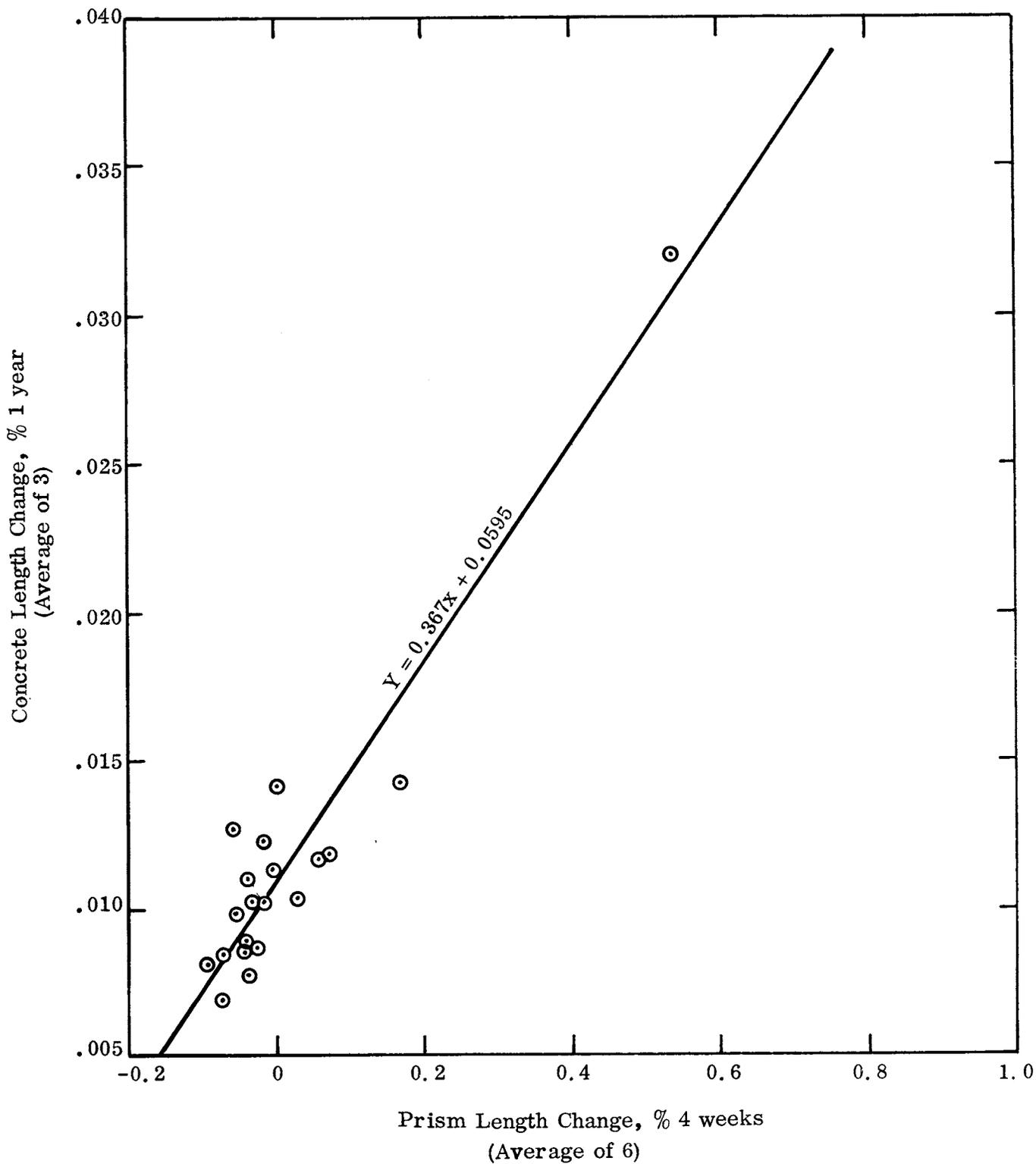
Figure 11. Concrete vs. prism length change.
