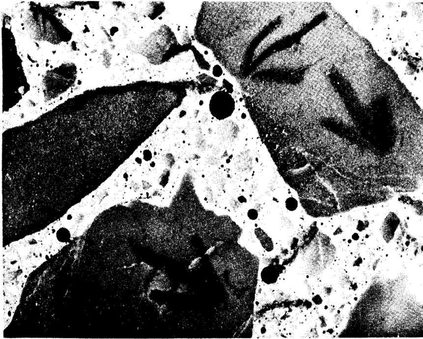
Figure 15. Aggregate 12-9 with high alkali cement. Expansion of concrete after 1 year equals 0.096%. Primary features are cracks in aggregates, cracks in aggregates extending into the mortar and very minor rims on aggregates. (3x)
