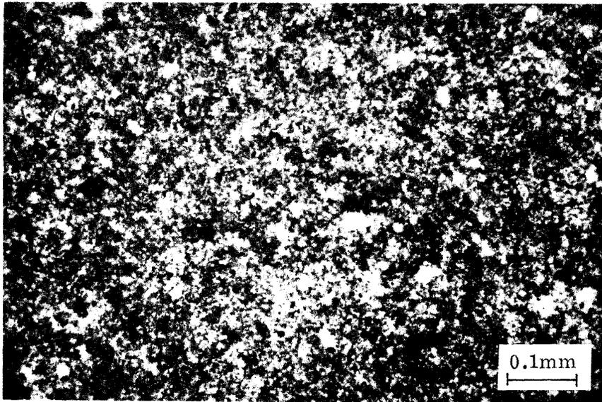
Figure 20. Texture of aggregate 5-1 representing material in prisms that did not expand. (125x)
