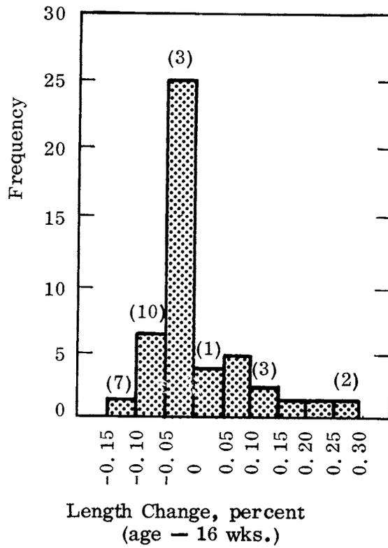
Figure 32. Distribution of length changes for prisms from Quarry 11 in the same form as shown in Figure 30.
