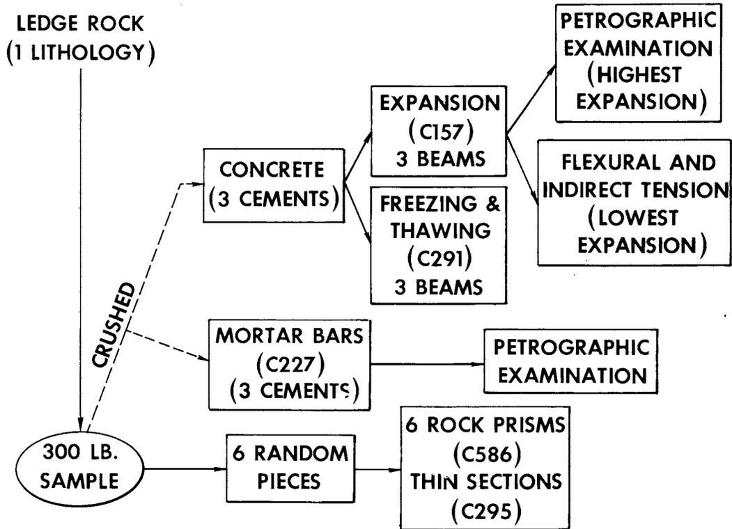
Figure 1. Schematic outline of testing program.
