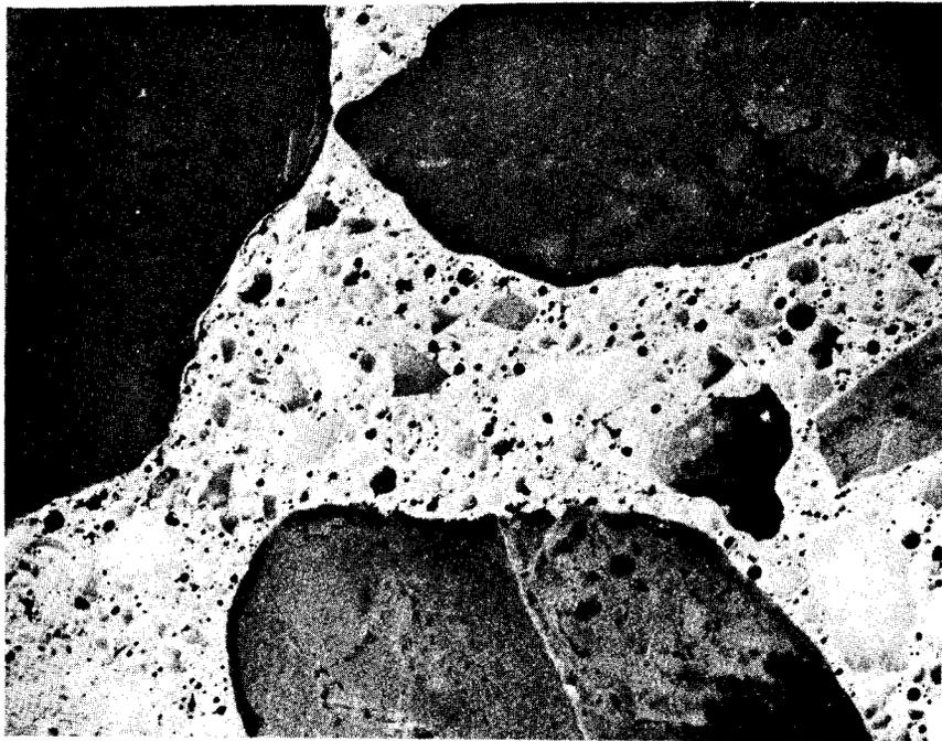
Figure 16. Aggregate 12-9 with medium alkali cement. Expansion of concrete after 1 year equals 0.086%. Primary features are slight boundary separation, cracks extending into the mortar and some rims on aggregates. (3x)
