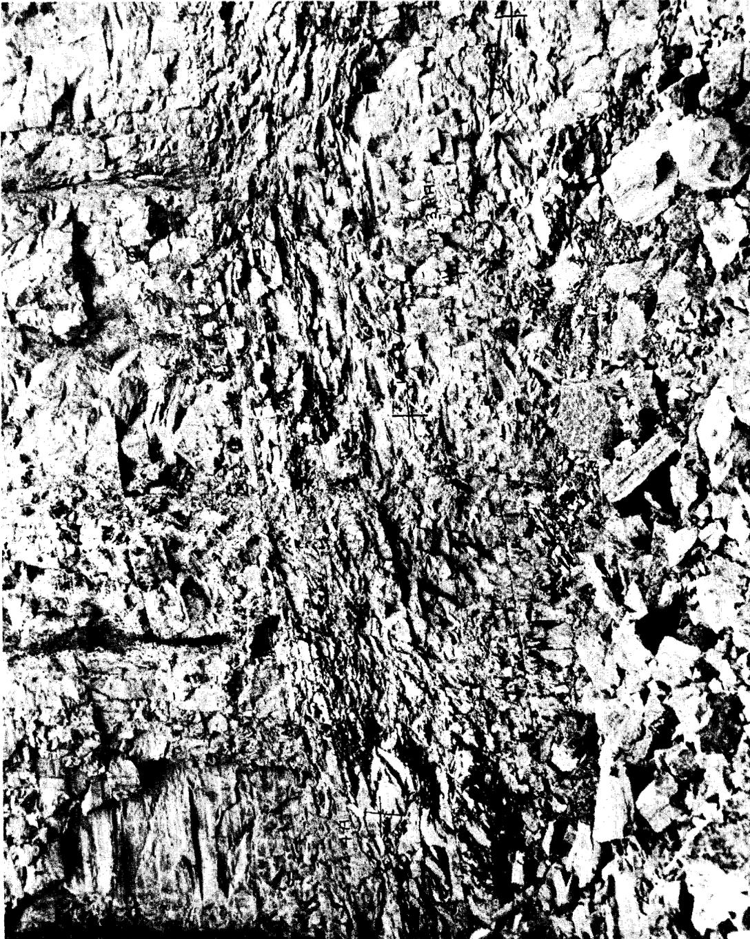
Figure 39. Another face of Quarry 12 illustrating the close proximity of highly expansive and non-expansive rocks.
