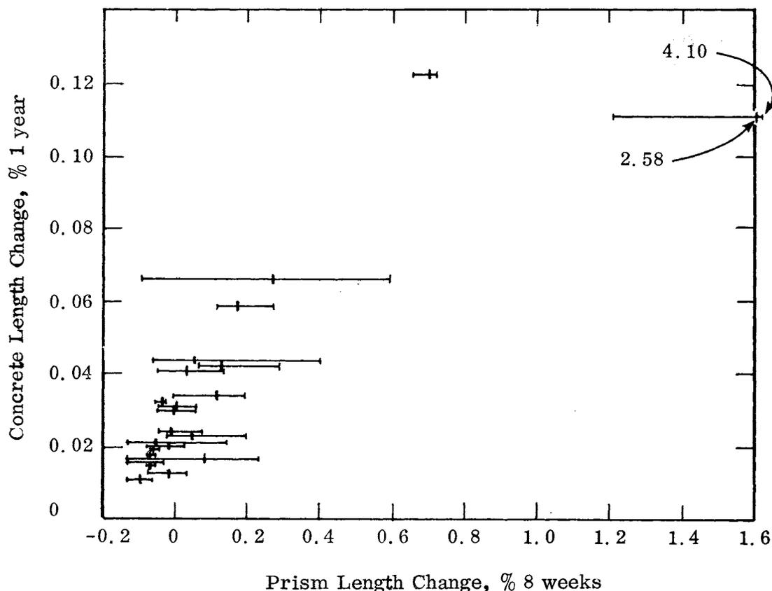
Figure 10. Relationship between length change at 1 year of concrete containing high alkali cement and length change of prisms at 8 weeks. Average and range of prism length change are shown for each sample.
