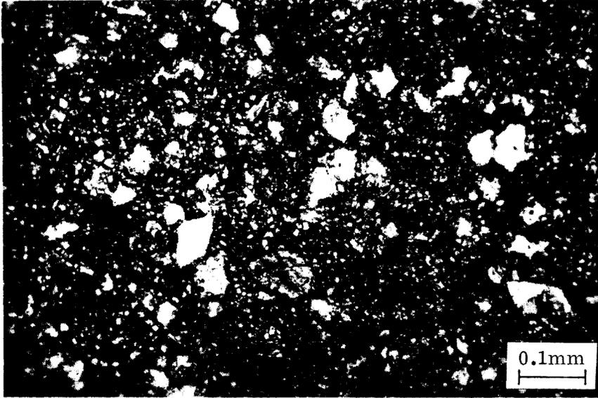
Figure 28. Texture of aggregate 13-1 that showed delayed expansion in prisms but no expansion in mortar bars or concrete.
