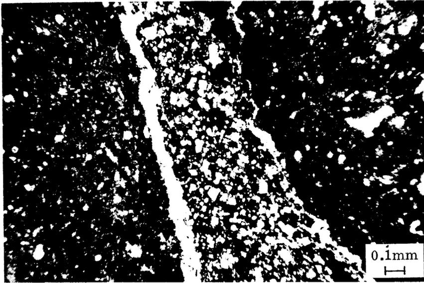
Figure 22. A vein of reactive texture in aggregate 11-X enclosed by an innocuous texture. (45x)
