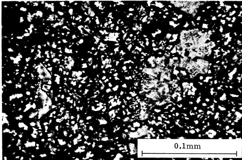
Figure 29. Close-up of texture of aggregate 13-1. (460x)
