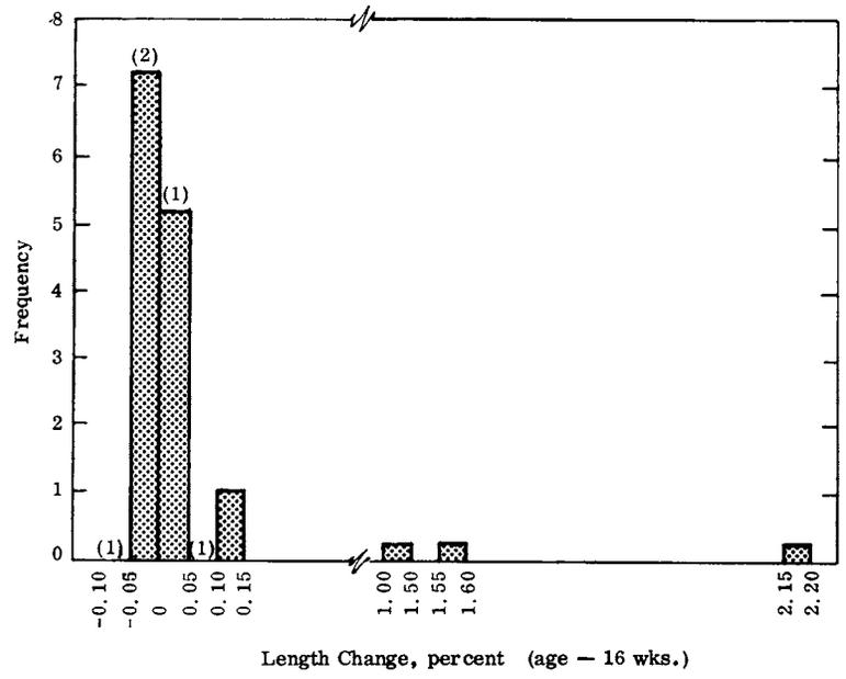
Figure 36. Distribution of length changes for prisms from Quarry 48 in the same form as shown in Figure 30.
