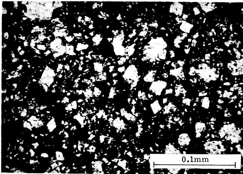
Figure 18. Classical reactive texture as seen in thin sections of aggregate 1-8. (380x)
