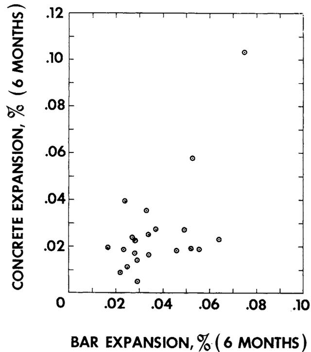
Figure 13. Mortar bar vs. concrete expansion (6 months).
