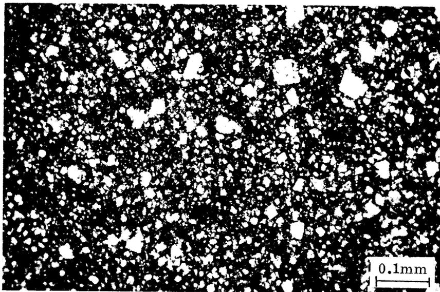
Figure 21. Texture of aggregate 5-1 representing material in concrete beams that expanded. (125x)
