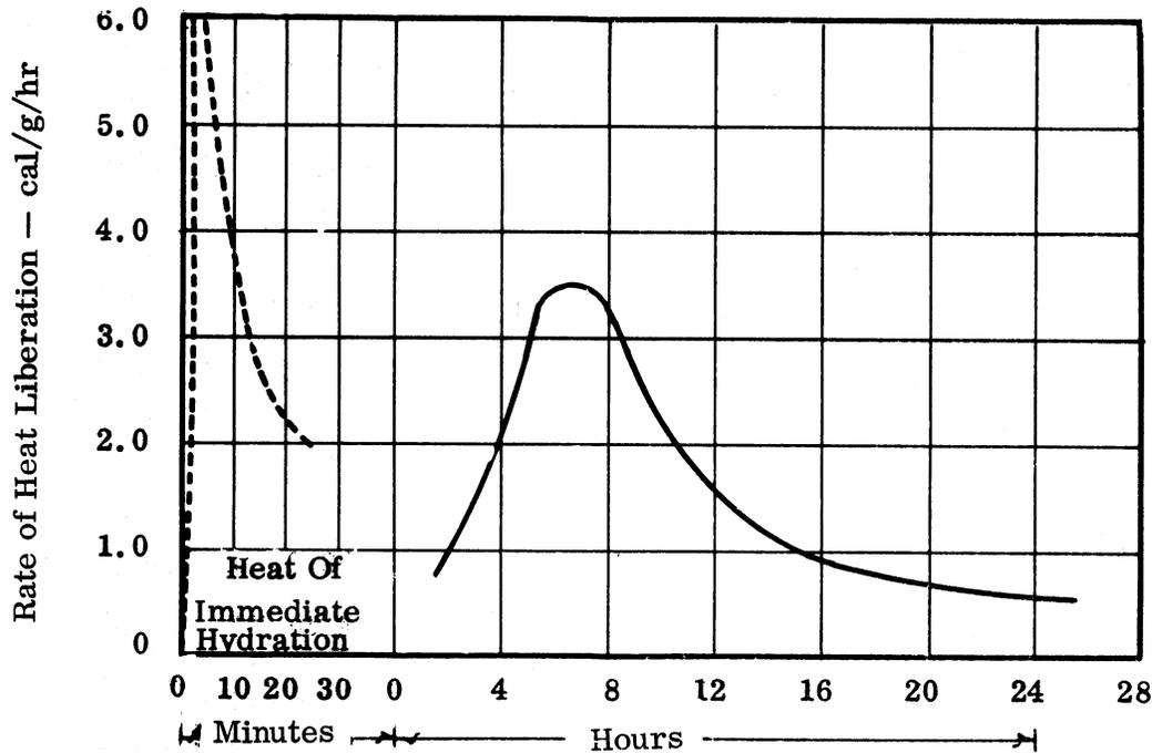
Figure 1. Rate of hydration of a typical cement with a proper  $\text{SO}_3$  content. After Lerch. (5)
