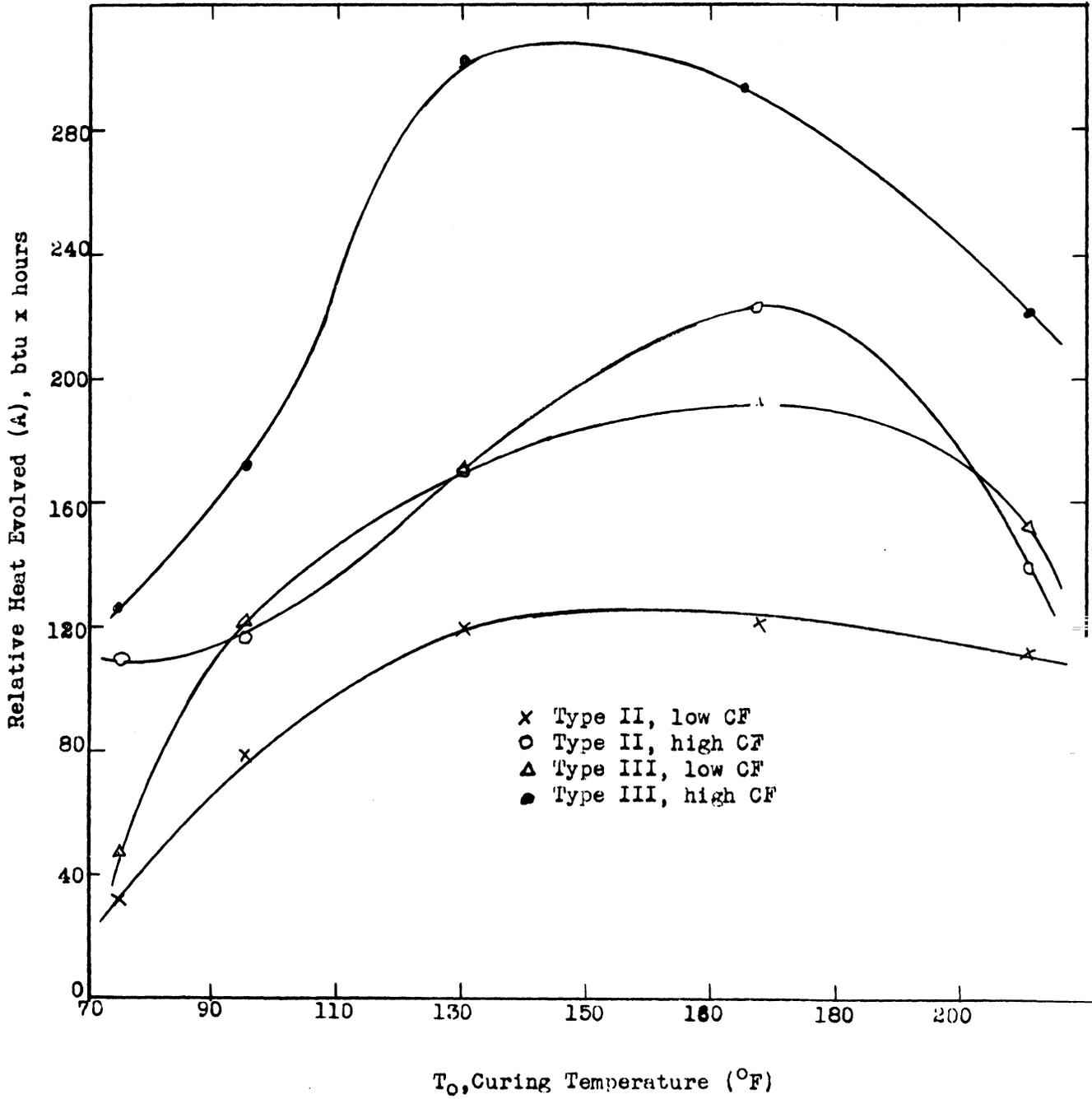
Figure 12. Relative total amounts of heat involved versus curing temperature.
