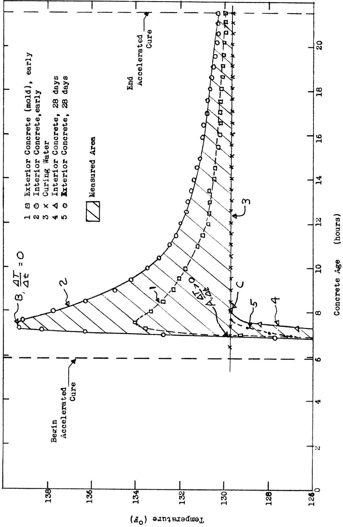
Figure 10. Typical time-temperature history for concrete during accelerated curing. Type III cement, high cement factor,  $T_0 = 130^\circ \text{F}$ . curing.
