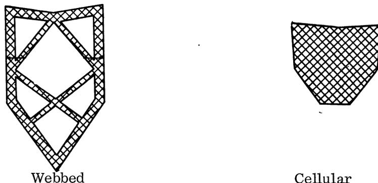
Figure 5. Preformed seal typical configurations.
