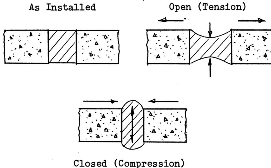
Figure 3. Behavior of poured joint sealant subjected to joint movement. After ACI Committee 504. (4)
