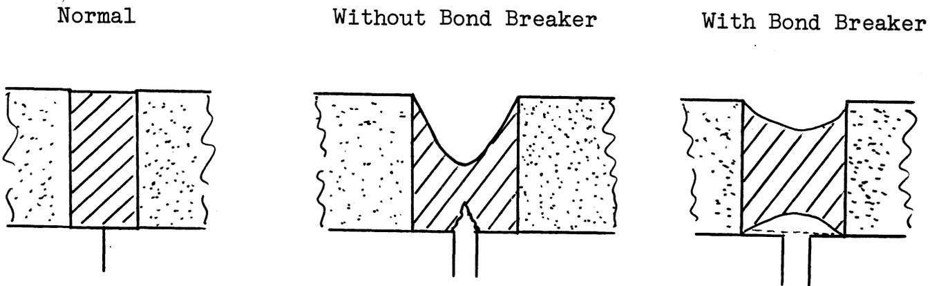
Figure 4. Sealant behavior with and without a bond breaker at the lower seal-concrete interface. After Schultz.<sup>(5)</sup>
