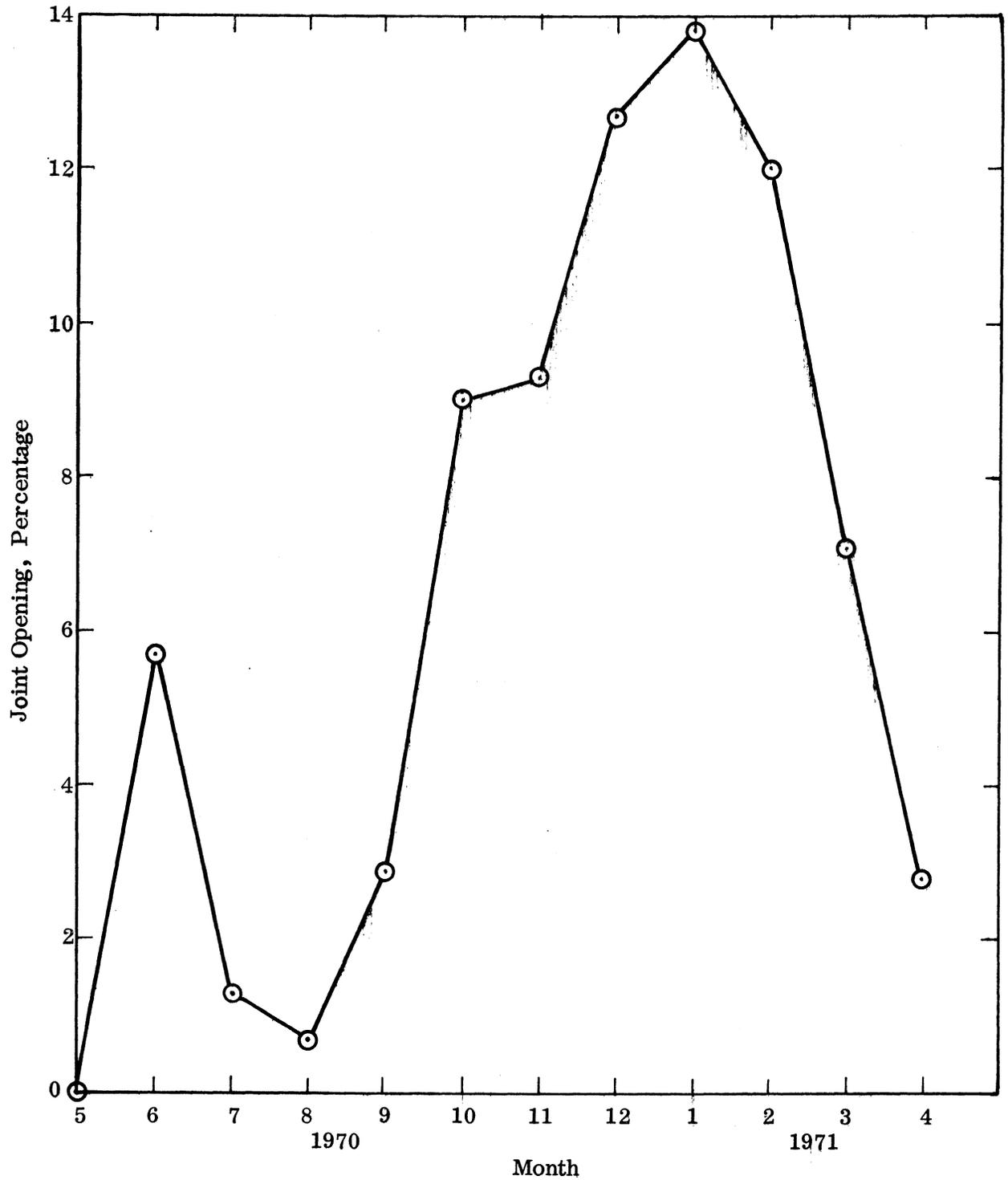
Figure 1. Seasonal variations in joint opening for typical joint on ramp pavement (20' joint spacing, 3/8" joint), I-64 near Charlottesville.
