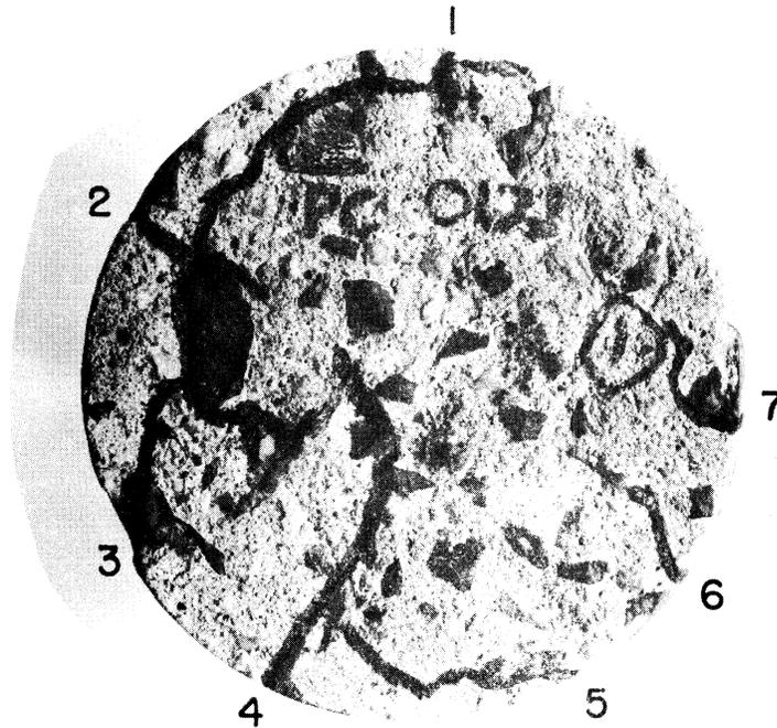
**Figure 8.** Top slice of core from scaled and pattern cracked area in northern project. Note exposed coarse aggregate (dark gray to black) and cracks (outlined in ink) across core and alongside coarse aggregate particles.
