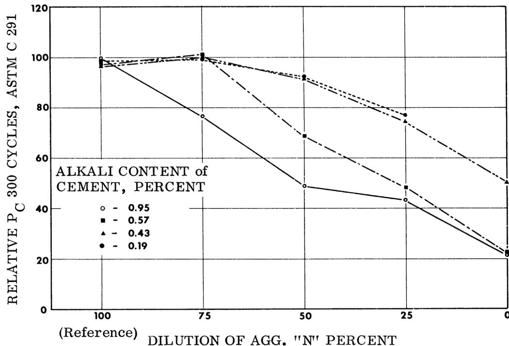
Figure 20. Freeze-thaw durability of dolomitic limestone (Aggregate 'N') with varying concentrations of granite reference aggregate and varying percentages of alkalis.
