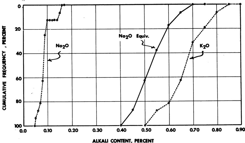
Figure 1. Alkali contents of cements used during the period of construction of bridges in both the northern and southern projects.
