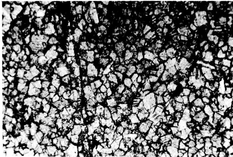
Figure 6. Typical view of crystalline dolomite. Explanation in text. Field is 1.3 mm. plane polarized light.
