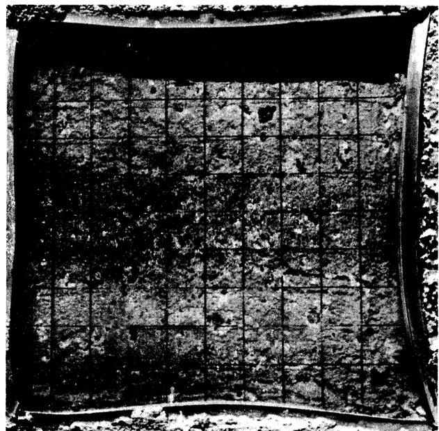
Figure 19. Age 14 months, northern aggregate, med-low alkalis, 4.4% air,  $\text{NaCl}$  treatment — compare with Figure 18.
