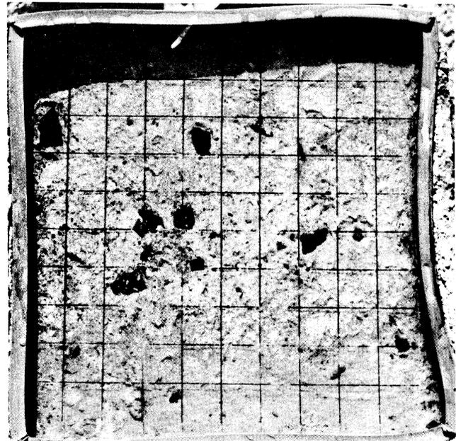
Figure 17. Age 14 months, northern aggregate, med-low alkalis 4.9% air,  $\text{CaCl}_2$  treatment — compare with Figure 16.
