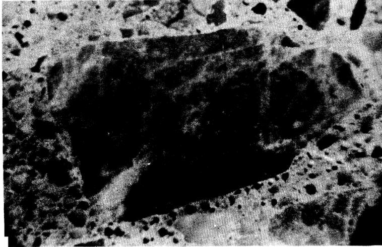
Figure 7. Detail view of coarse aggregate particle from southern project in cut and polished surface. Note internal fractures and veins in particle.
