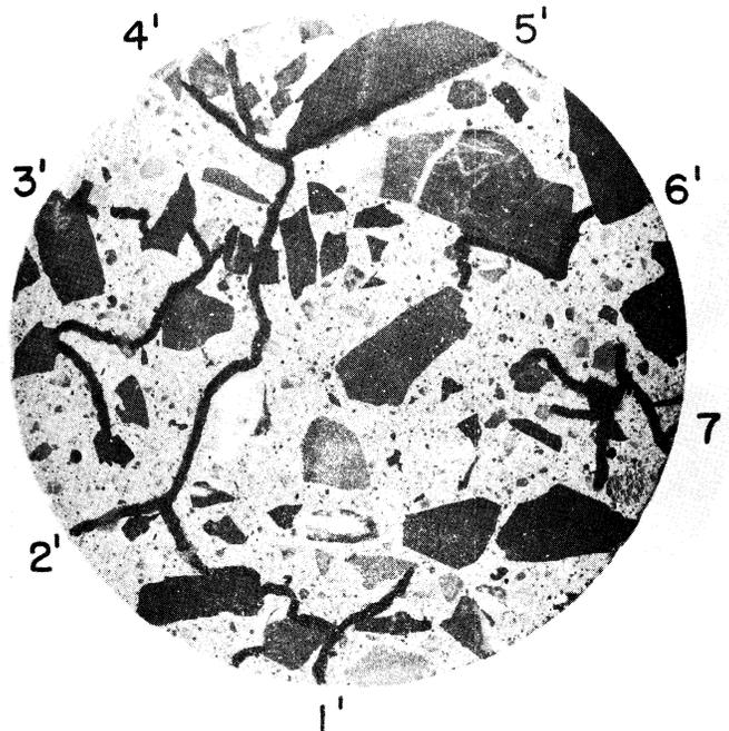
**Figure 9.** Interior polished underside of core shown in Figure 8 showing same crack pattern as pavement surface. Cracks corresponding to those numbered in Figure 8 are evident.
