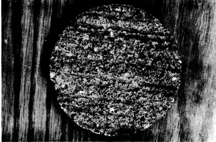
Figure 5. Typical view of pavement surface of core from southern project. Note finishing marks still visible.
