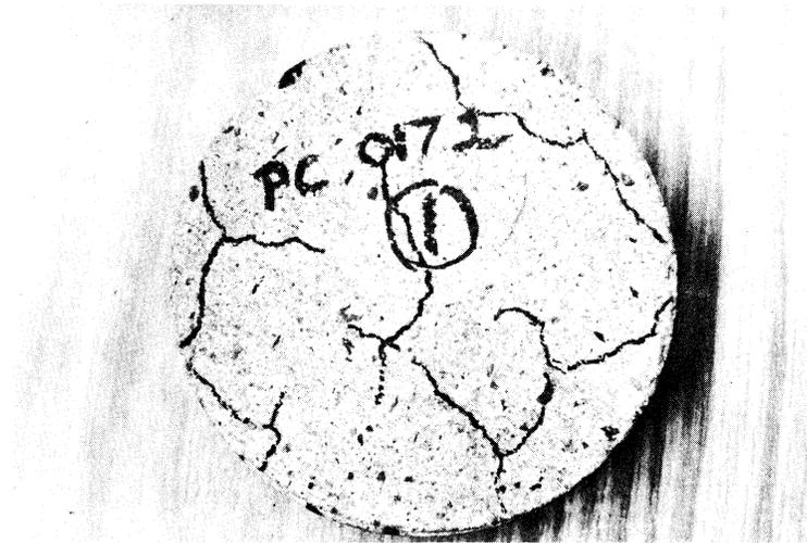
Figure 11. Core from location in Figure 10 showing system of hairline cracks which have been outlined in black.
