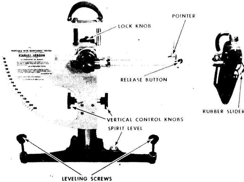
Figure 8. British Portable Skid Resistance Tester.
