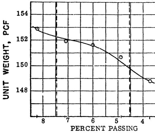
Stability and Volumetric Properties Resulting From Variations in Percent Passing the No. 200 Sieve
