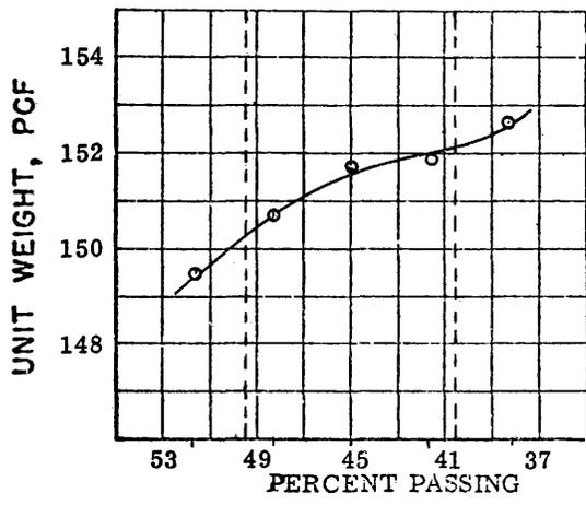
Stability and Volumetric Properties Resulting From Variations in Percent Passing the No. 8 Sieve
