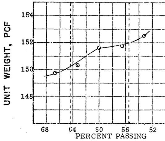
Stability and Volumetric Properties Resulting From Variations in Percent Passing the No. 4 Sieve
