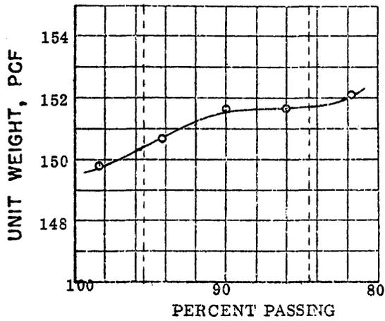
Stability and Volumetric Properties Resulting From Variations in Percent Passing The 3/8" Sieve
