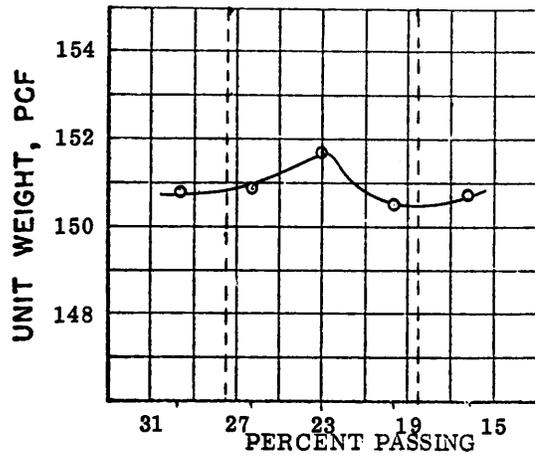
Stability and Volumetric Properties Resulting From Variations in Percent Passing the No. 30 Sieve
