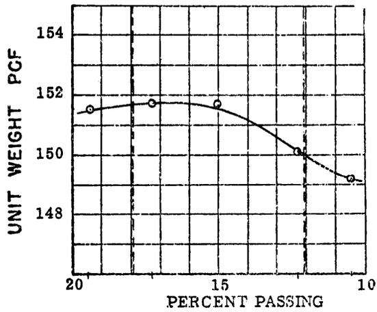
Stability and Volumetric Properties Resulting From Variations in Percent Passing the No. 50 Sieve
