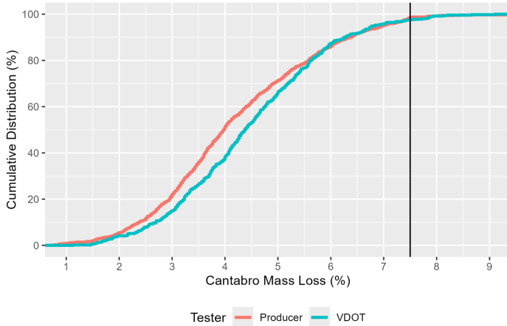
Figure 7. Cantabro Mass Loss Production Results (Maximum Passing Threshold of 7.5% Mass Loss)
