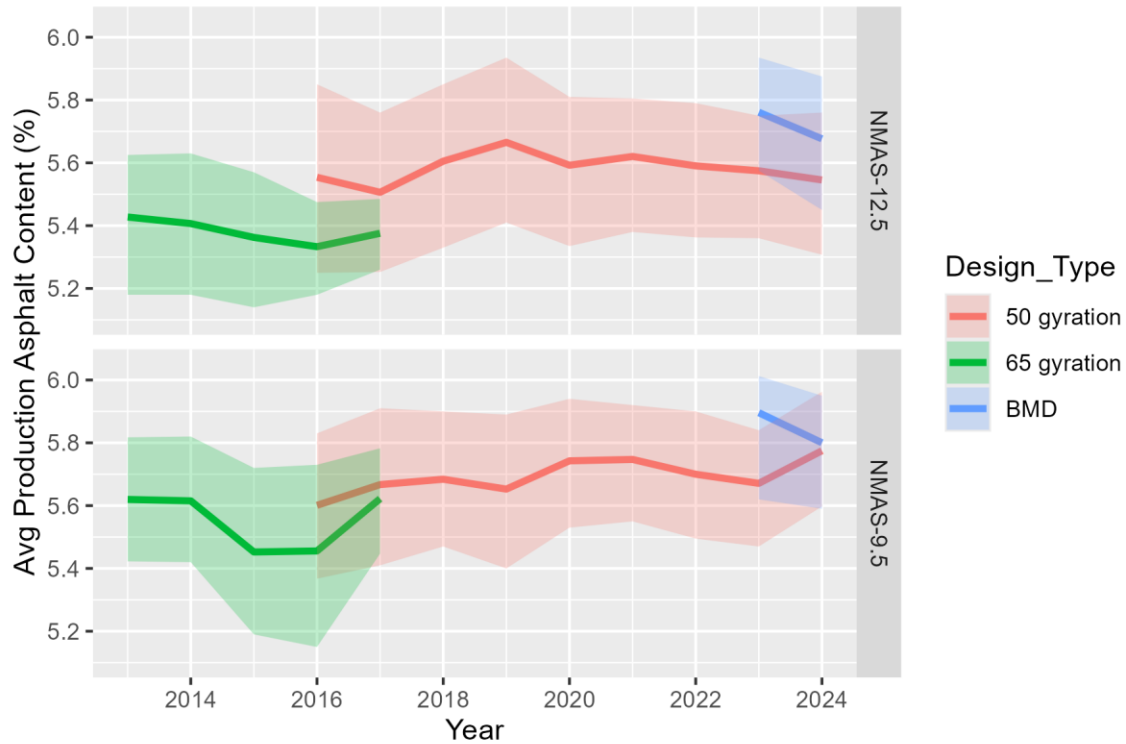
Figure 6. Average Production Asphalt Content by NMA and Mixture Design Method. Shaded area indicates 25th and 75th percentile values. BMD = balanced mix design; NMA = nominal maximum aggregate size.
