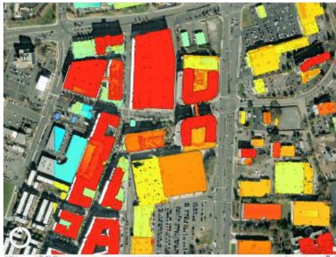
Figure 11. LiDAR Point Clouds in Figure 4 Classified as Buildings. Imagery copyright of the Commonwealth of Virginia, Maxar, and Microsoft. LiDAR = light detection and ranging.
