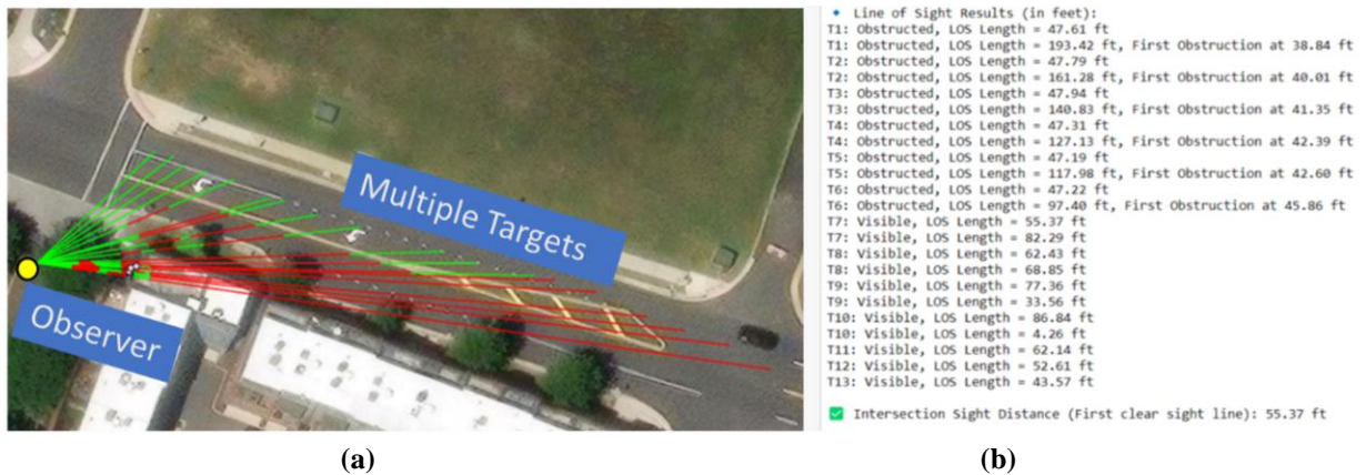
Figure 12. (a) Example of Line of Sight Analysis with Multiple Targets from an Observer Point; (b) Python Script Output. Imagery copyright of the Commonwealth of Virginia, Maxar Technologies, and Microsoft.
