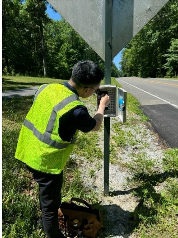
Figure 46. Manual Rebooting People Counter at Location #1
