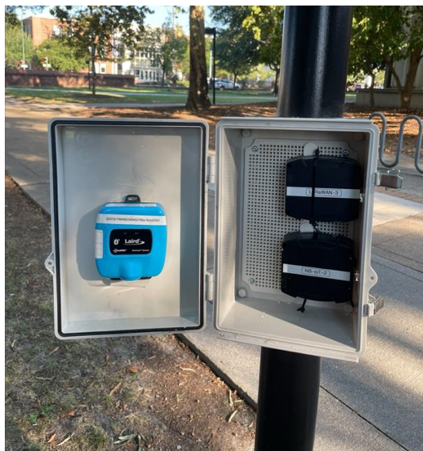
Figure 12. A Laird Temperature Sensor, a LoRaWAN People Counter, and an NB-IoT People Counter Housed in A Waterproof Enclosure, Mounted on a Light Pole at ODU's Norfolk Campus
