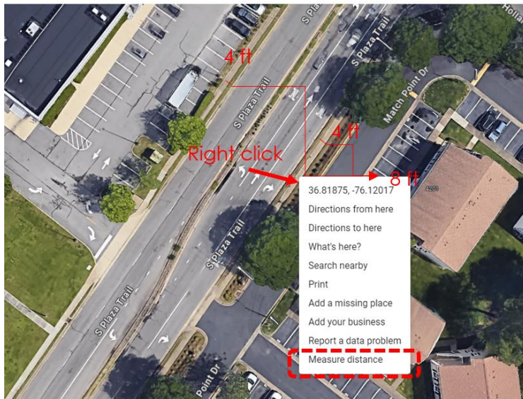
Figure D6. Determine the Total Width of the Sidewalk on Both Sides, Map Data ©2023 Google
