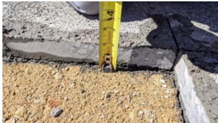
**Figure 38. Confirmation of the thickness of the paved asphalt sections**
