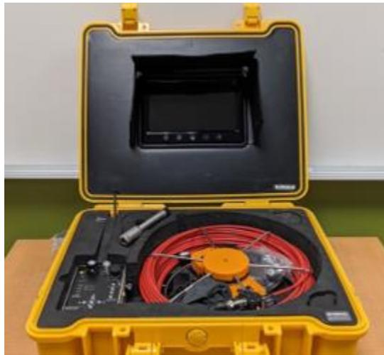
**Figure 16. The instrument used to survey the edgedrain and collection pipes at each section**
