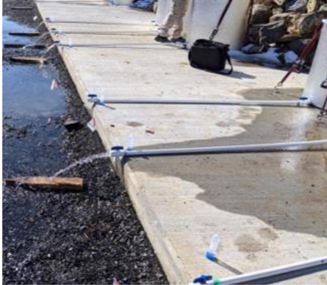
**Figure 7. Water sampling pipes from the collection tanks**
