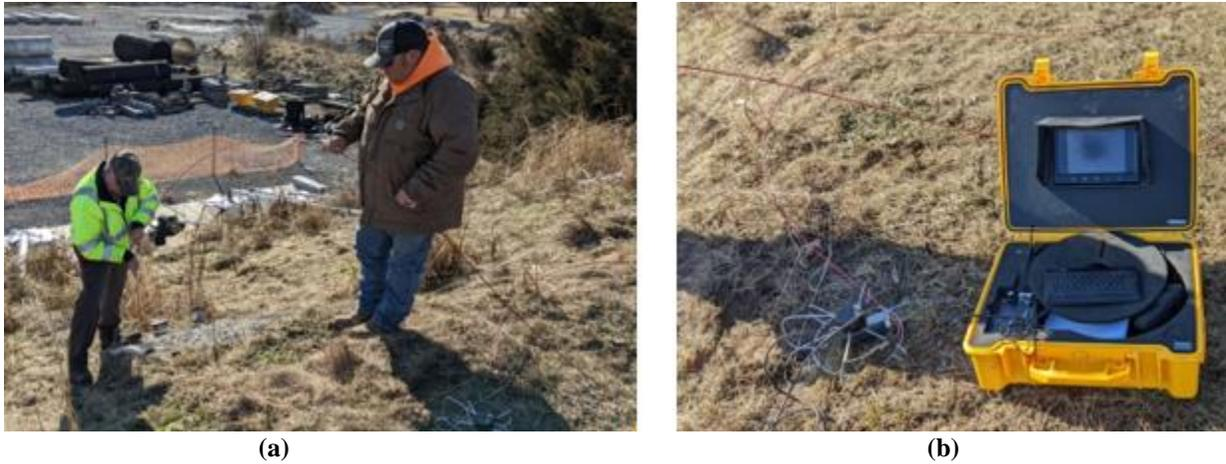
Figure 17. Insertion of the (a) borescope camera through the T connector and (b) monitoring and data collection on site
