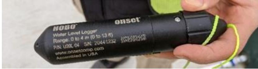
**Figure 5. Water level logger installed at each collection tank**
