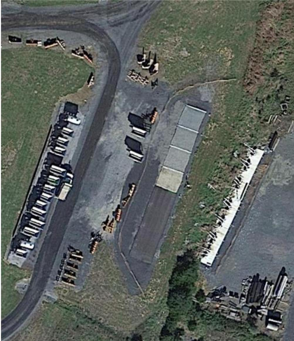
**Figure 26. A Google earth© photo of the completed test site showing the locations of the three paved and four unpaved sections and the collection water tanks adjacent to the site located downslope**
