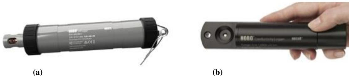
**Figure 6. The (a) pH and (b) electric conductivity (EC) logger sensors installed into the water collection tanks of the 100% unpaved CHCC test section**
