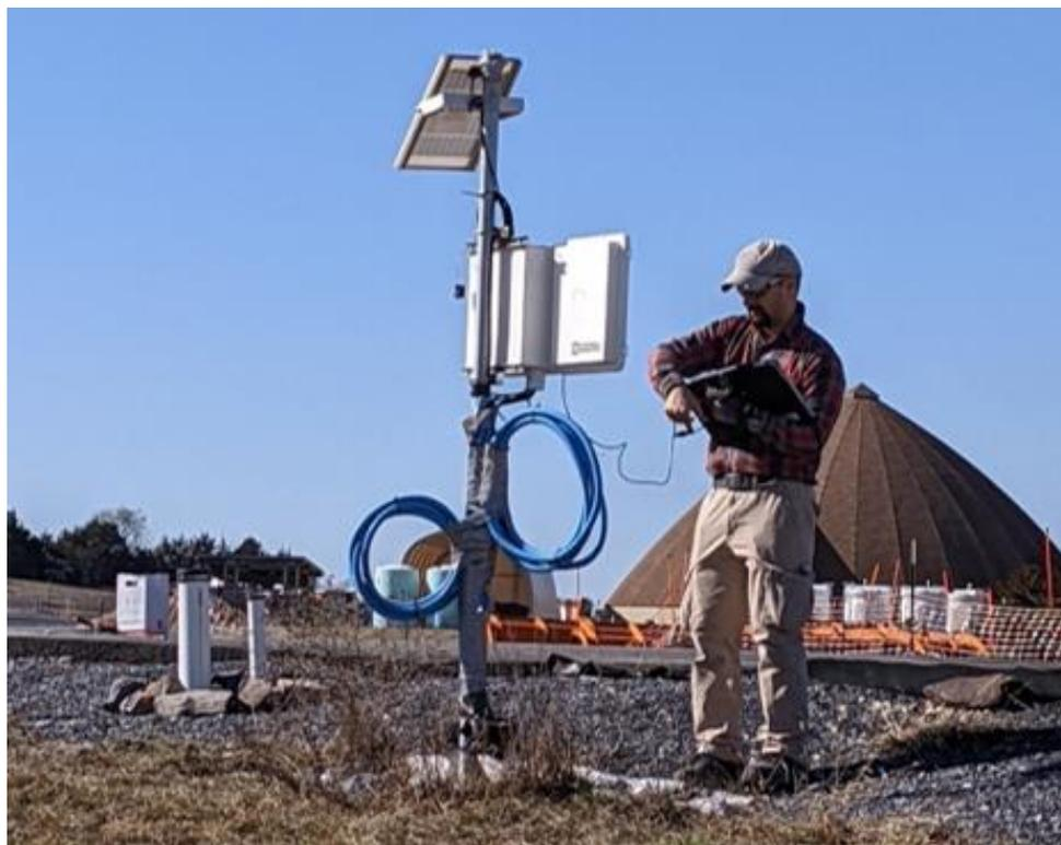
**Figure 4. The data logger pole for all sensors installed within the base course at the test site**
