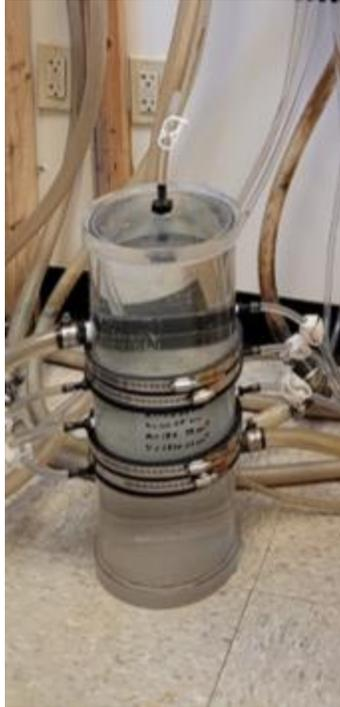
**Figure 13. Evaluating the permittivity of the geotextiles exhumed from the test site**
