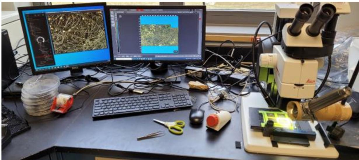
**Figure 15. The Leica M125 C microscope with an in-built 5 MP HD digital camera with a geotextile sample under analysis**
