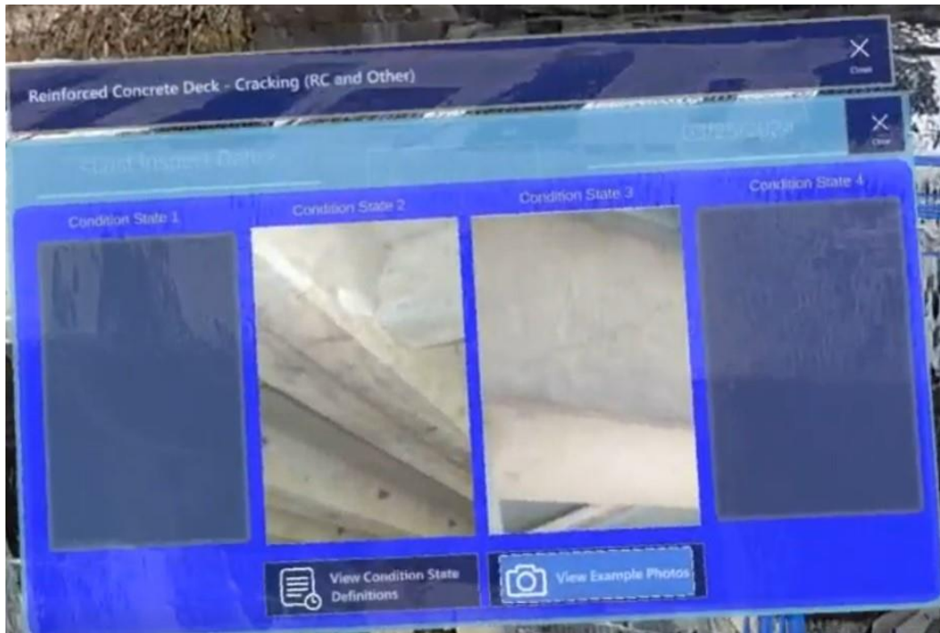
Figure 26. Shows example photos provided when “View Condition State Details” is chosen in the context of Reinforced Concrete Deck – Cracking (RC and Other). Photos obtained from the AASHTO Bridge Reference Manual.
