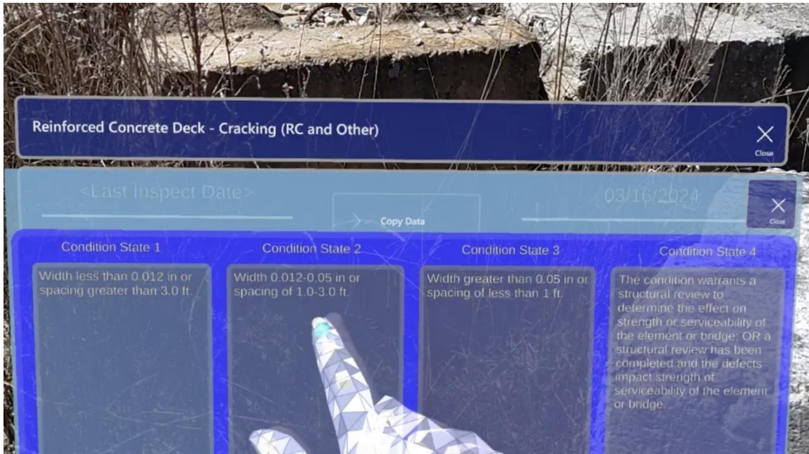
Figure 25. Example of information displayed when “View Condition State Details” is chosen in the context of a Reinforced Concrete Deck – Cracking (RC and Other).
