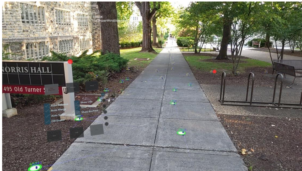
Figure 28. Test on Virginia Tech campus of the World Locking Tools system to see the average tracking error (virtual object drift) incurred over around 1,100 feet of Straight-line headset movement tracking.
