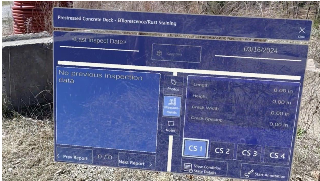
Figure 19. Defect data panel. Note that the menu title is incorrect: It should read Cracking (RC and Other), as this relates to the available data entry options.
