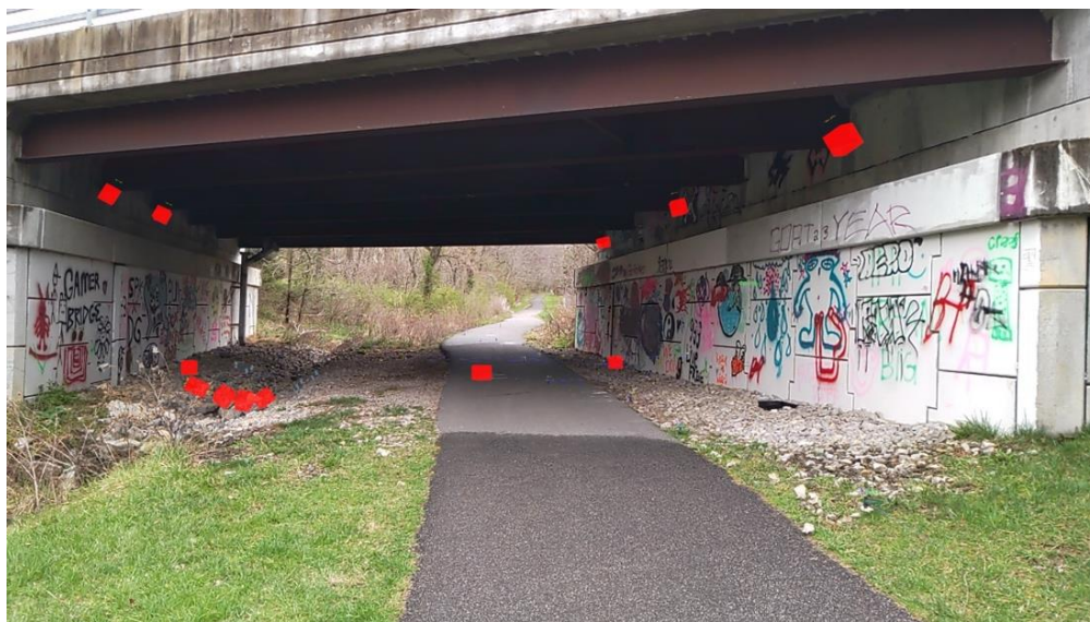
Figure 27. Virtual objects at Virginia Tech test bridge used to ensure the persistence of virtual objects in the tracking system.
