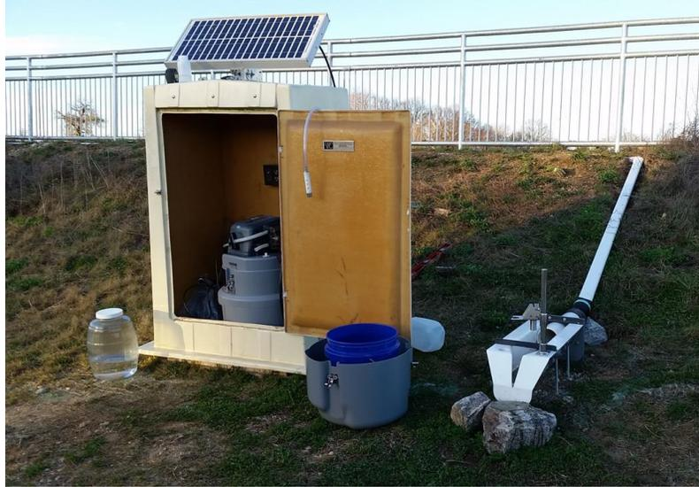
**Figure 3. Stormwater sampling setup at the roadside sheet flow collector along Lorton Road**
