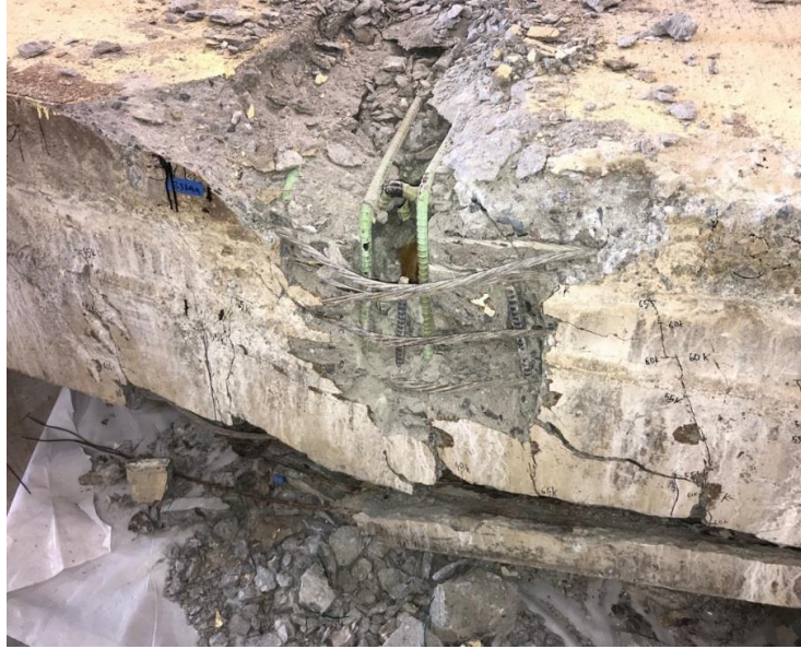
Figure 72. Crushing of the Top Flange of Box Beam 2
