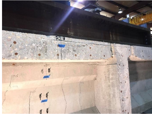
Figure 55. Crushing of Top Flange at Failure of I-Beam 3
