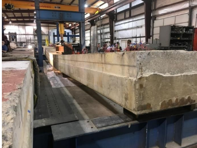
Figure 74. Large Displacement of Box Beam 2
