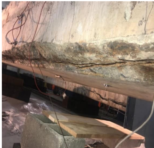
Figure 75. Corroded Strand on Bottom of Box Beam 2
